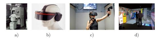
Figure 2.17 – From left to right several virtual reality devices through time with: Sensorama (a) in 1956, SegaVR (b) in 1991, Vive (c) in 2019 and Immersia Cave (d) in Rennes
