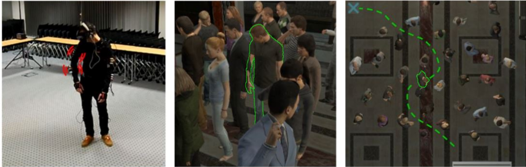
Figure 6.1 – Our objective is to understand whether and to what extent providing haptic rendering of collisions during navigation through a virtual crowd (right) makes users behave more realistically. Whenever a collision occurs (center), armbands worn on the arms locally vibrate to render this contact (left). We carried out an experiment with 23 participants, testing both subjective and objective metrics regarding the user’s path planning, body motion, kinetic energy, presence, and embodiment.
