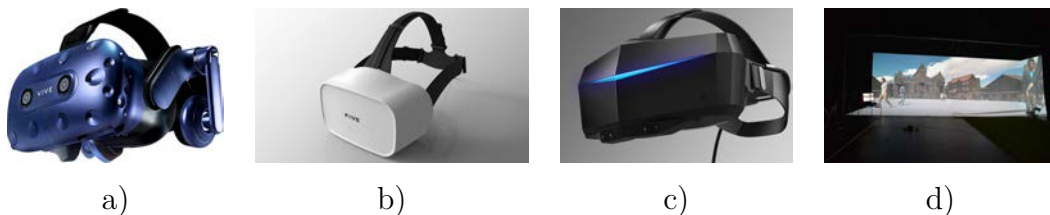
Figure 3.6 – From left to right list of virtual reality devices supported by CrowdMP: HTC Vive (a), Fove (b), Pimax (c) and Immersia (d).
