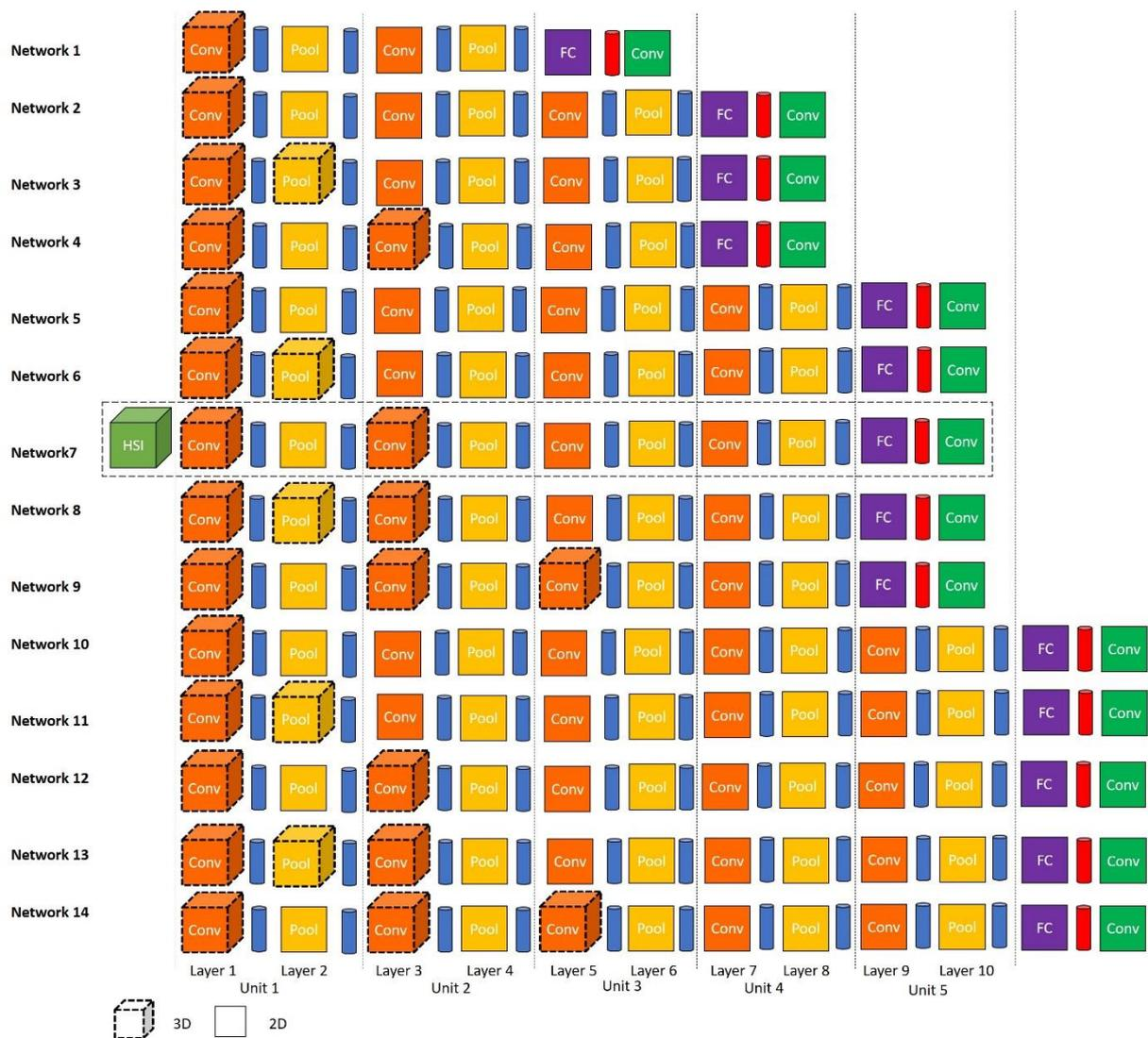
Supplementary figure 7: All the fourteen structures tested in the optimization step with 3D and 2D layers, and 4 to 10 layers
