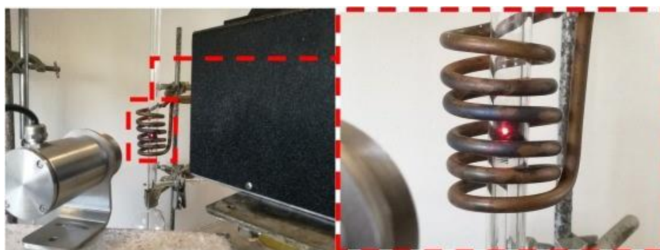
Fig. 1. Digital photos of the Ni/OCF catalyst in the quartz tubular reactor placed inside the coils of the inductive heater along with the laser pyrometer for the control of the temperature inside the catalyst bed.
