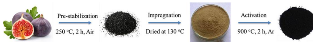
Fig. 2-1. Schematic of synthesis procedures of hierarchical carbon structure from waste fig fruit.
