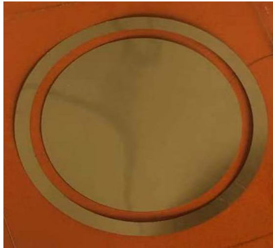
Figure 3.13 PI film view and guard ring gold electrode deposition
