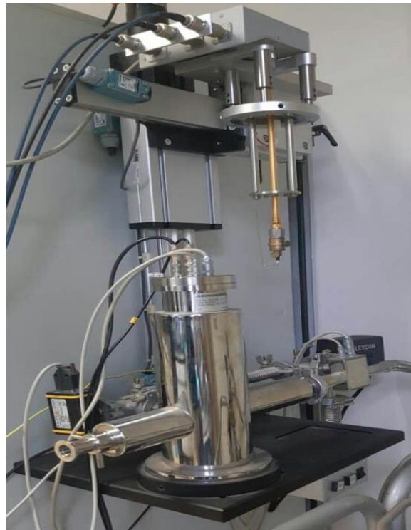
Figure 3.22 TSC measuring system electrode
