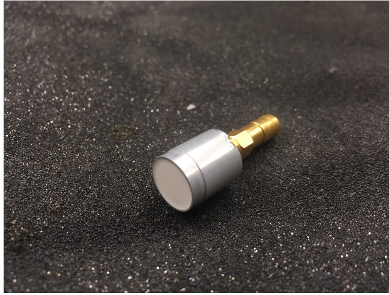
Fig. IV.5 Image of the ultrasound transducer used in the experiment. Diameter of the transducer is 12 mm and has emitting frequency of 230 kHz.
