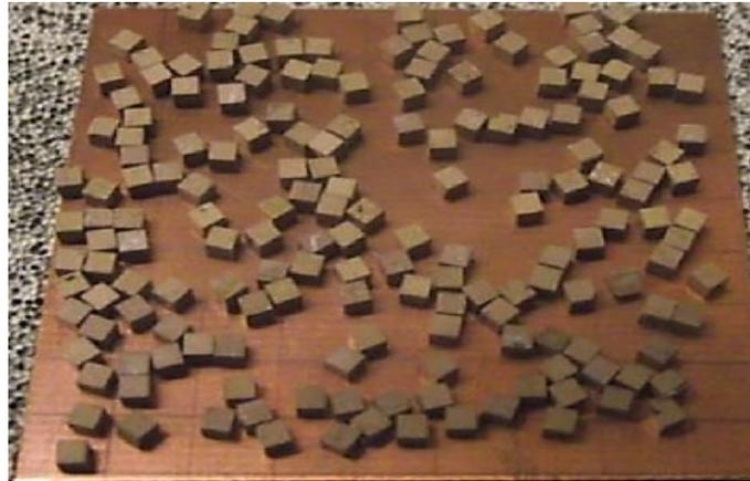
**Figure 1.15:** Photograph of the random BST cubes sample deposited on the copper plate [57].
