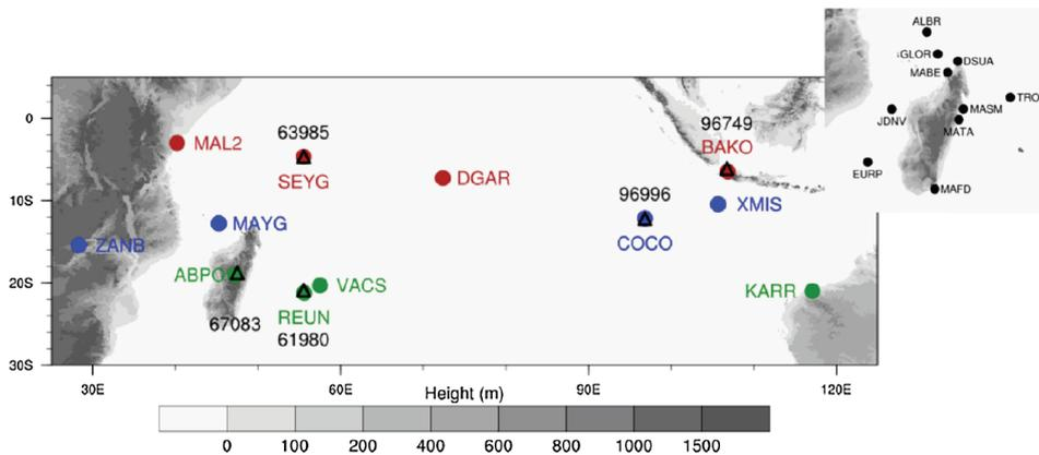
**FIGURE 1** Location of the twelve IGS ground-based GNSS stations (circles) and the five radiosonde stations (triangles) used in this study. Insert shows the locations of new GNSS research stations recently deployed in the southwest Indian Ocean basin in the framework of the Indian Ocean GNSS Applications for Meteorology (IOGA4MET) research program. Red, blue and green colours indicate the three transects discussed in Section 3
