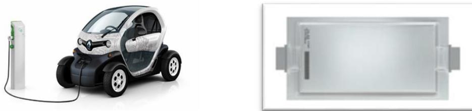
FIGURE II- 1: RENAULT TWIZY VEHICLE AND 43AH POUCH CELL.
