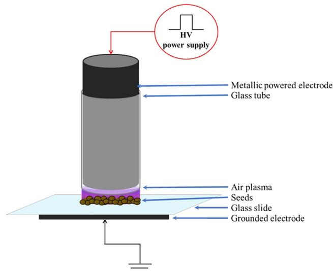
**Figure 1.** Scheme of the plasma device of dielectric barrier discharges (DBD) in ambient air. Interior glass tube diameter: 8 mm; glass slide thickness: 1 mm; metallic powered electrode diameter: ~8 mm.
