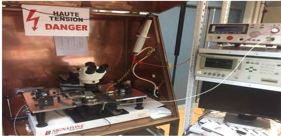
Figure 2-14. Breakdown testing experimental set-up
