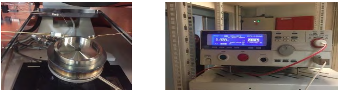
Figure 2-13. Signatone S-1160 probe station (left) and the electrical safety tester FI 9035HT (right)
