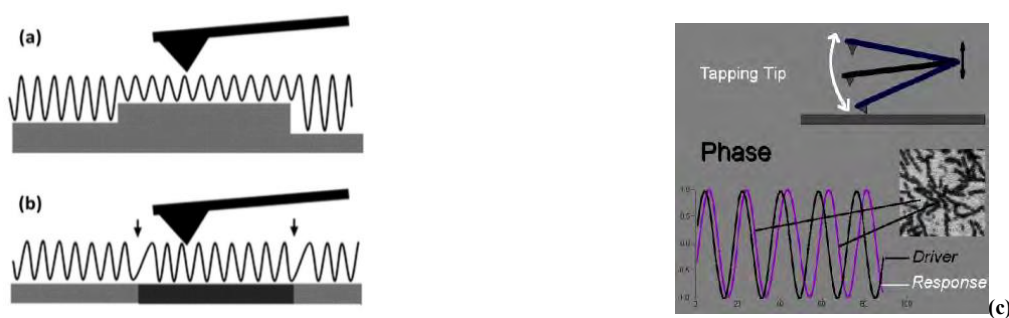
Figure 2-18. Schematic representation of the tapping mode: (a) the change in amplitude of oscillation is induced by the topography change, (b) the modification of the material properties introduces a phase shift of the oscillation (indicated in the figure by the arrows). (c) Phase shift over regions of different composition
