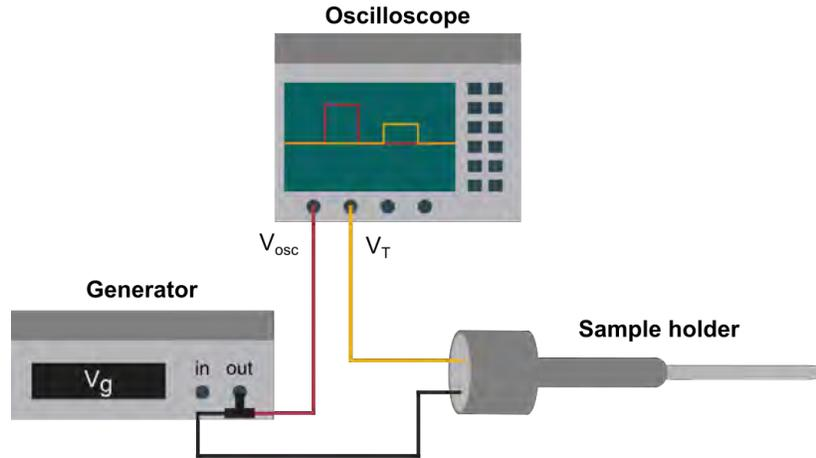
Figure 6.8: Schematics of the electronic setup used in the experiment.
