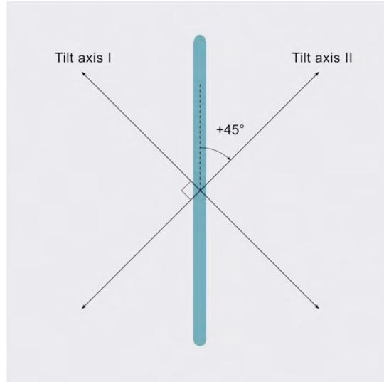
Figure 3.11: Illustration of a NW (green) lying on a carbon film of a TEM grid (gray). Two tilt axis with a  $90^\circ$  degree rotation with respect to each other, and with  $\pm 45^\circ$  relative to the NW axis are indicated by black double-headed lines.
