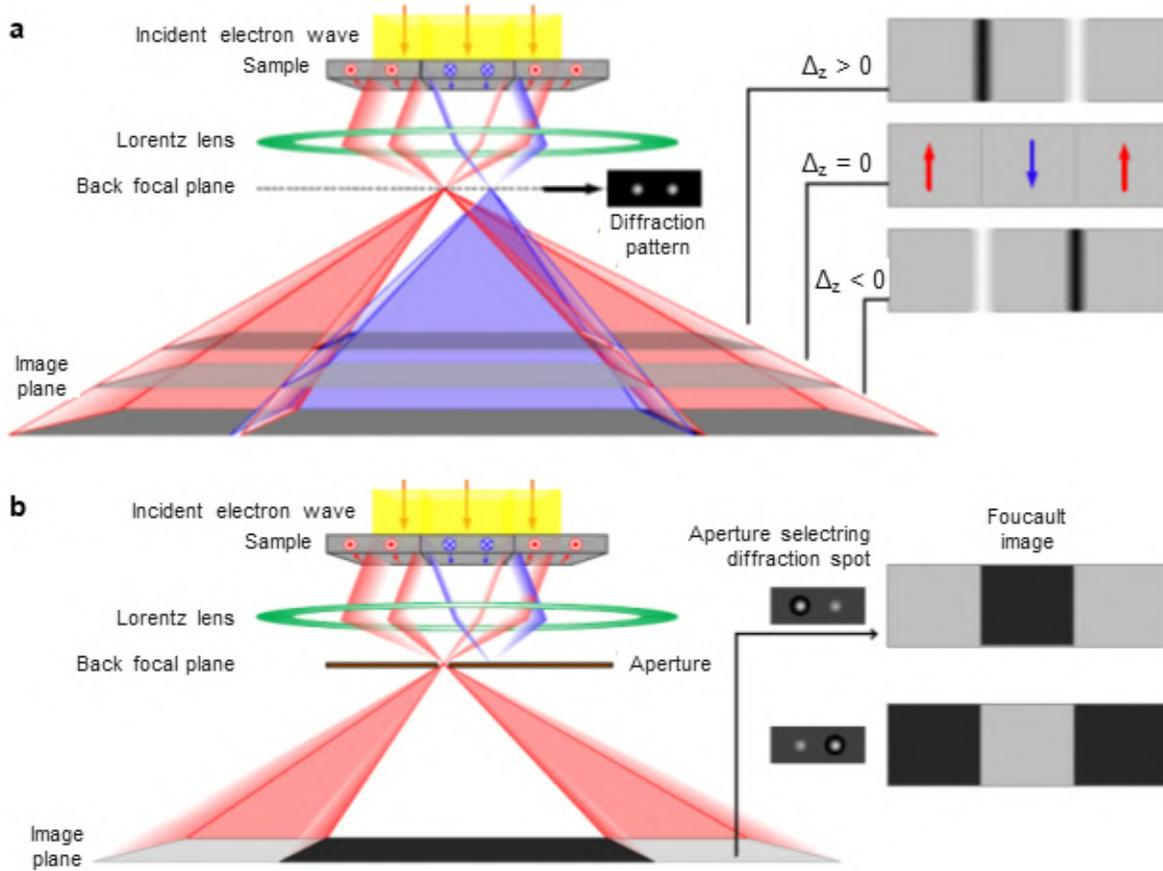
Figure 3.4: Illustration of the two Lorentz microscopy imaging modes: (a) Fresnel mode and (b) Foucault mode. The red and blue arrows in the sample represent the magnetization direction.<sup>8</sup>
