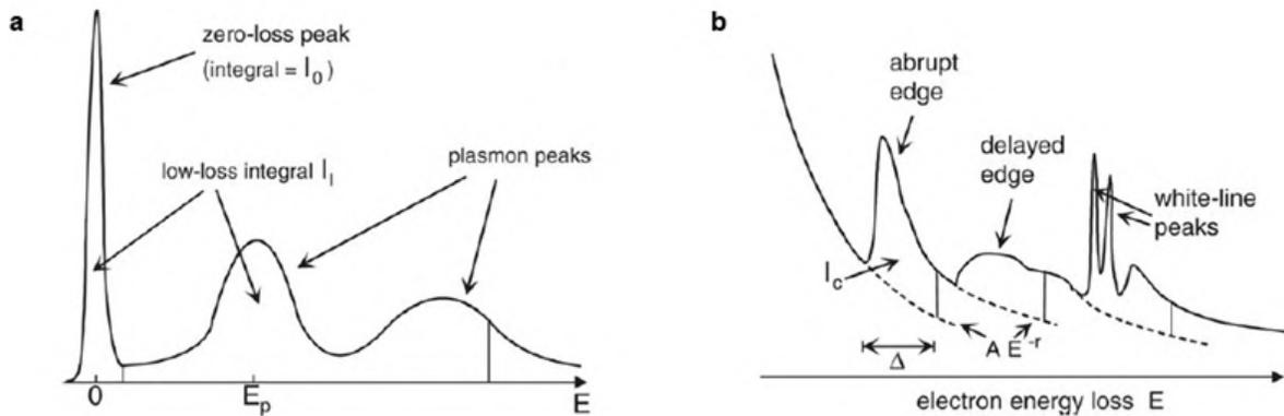
Figure 3.15: Figure showing typical EELS spectra: (a) show low-loss region and (b) show the core-loss region where the ionization edges are indicated together with their background, which is marked by the dashed line.<sup>46</sup>
