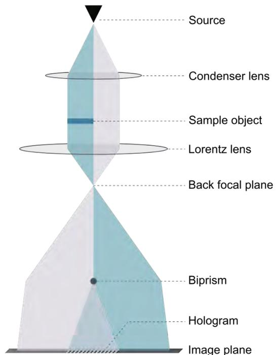
Figure 3.5: Principal TEM setup for off-axis electron holograph
