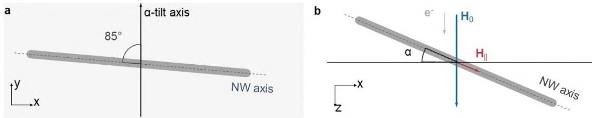
Figure 6.2: (a) Schematics showing the  $\alpha$ -tilt axis relative to the NW axis in the  $xy$ -plane. (b) Illustration of the field component applied parallel to the NW axis ( $\mathbf{H}_{\parallel}$ ) relative to the  $\alpha$ -tilt angle and the field applied by the objective lens ( $\mathbf{H}_0$ ).
