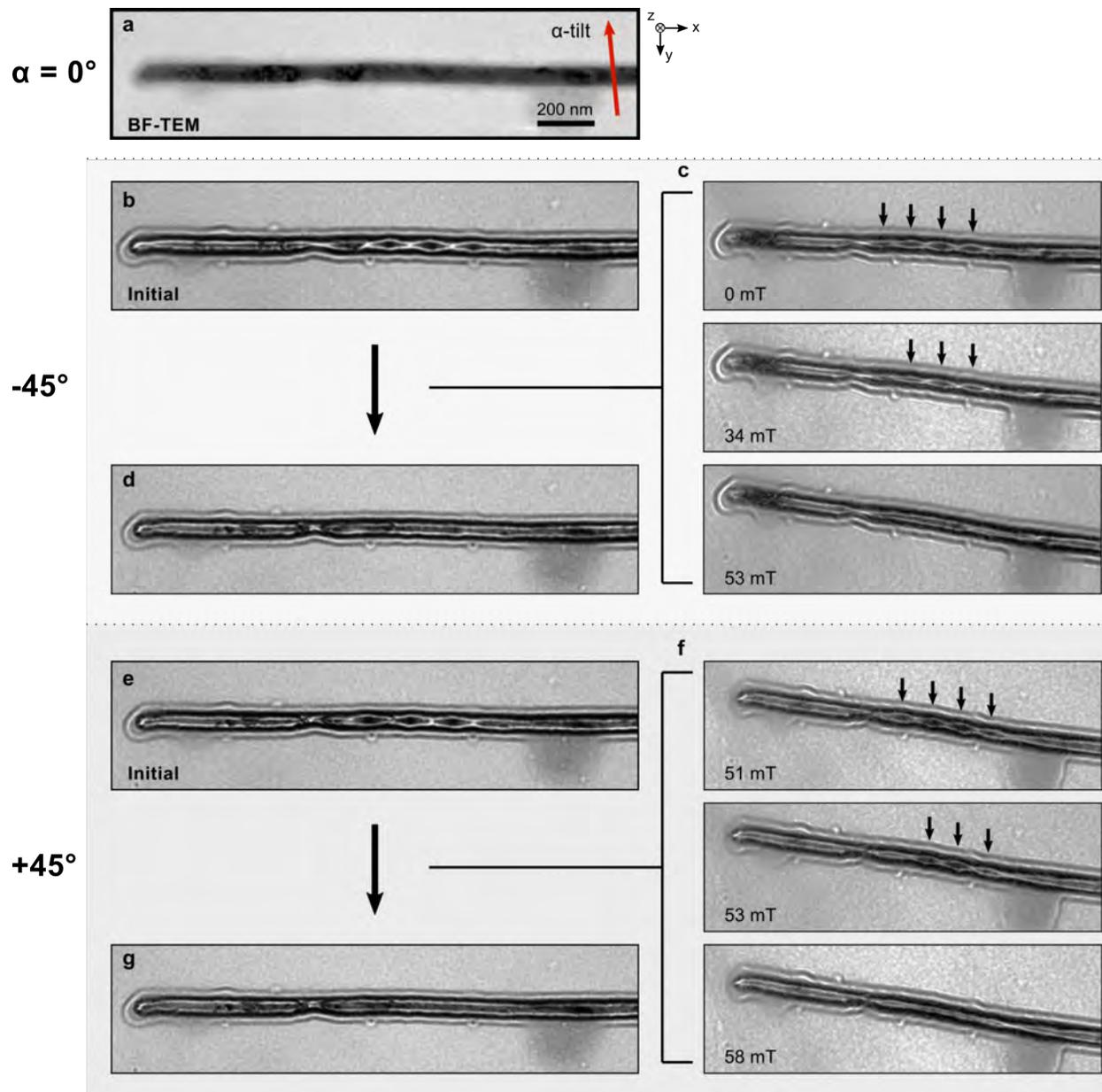
Figure 6.3: Results of *in situ* magnetic field application along the NW axis. (a) Bright-field TEM image of studied NW, where red arrow indicate the  $\alpha$ -tilt axis. (b)-(g) Fresnel images showing change in magnetic configuration from applied field along NW axis in both positive and negative  $x$ -direction by repeating the measurement at  $-45^\circ$  (b)-(d) and  $+45^\circ$  (e)-(g)  $\alpha$ -tilt.
