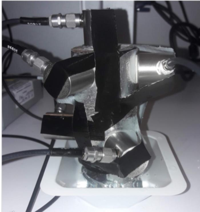
**Figure 5.6:** Photography illustrating a free capillary uptake in a sample prepared with Sodium Sulphate monitored with six PZTs attached with duct tape and communicating with Mistras acoustic system.
