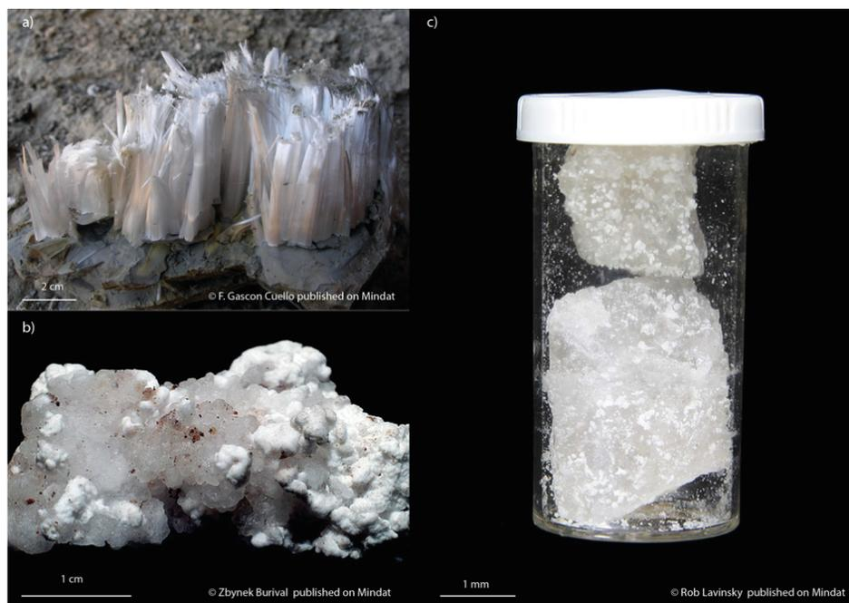
**Figure 2.12:** a) Fibrous crystal of epsomite b) Hexahydrate crystal partly dehydrate in whitish starkeyite c) Crystal of kieserite. Kieserite is stored in a waterproof box to avoid hydration in atmospheric conditions.
