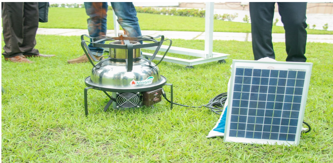
Photo 18 : Foyer hybride solaire-biomasse "Atingan"
