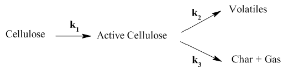
Figure 8: Broido–Shafizadeh model of cellulose pyrolysis.
