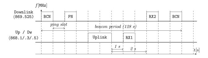
Figure 2.4: LoRaWAN Class B Transmission Schedule
