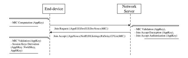
Figure 3.2: Join Procedure in LoRaWAN 1.0
