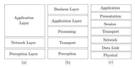
Figure 1.1: Different IoT Architecture models.
