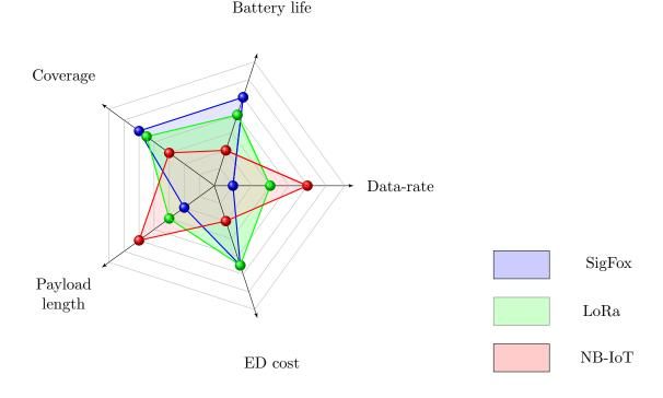
Figure 1.5: NB-IoT leading technologies comparison [2]
