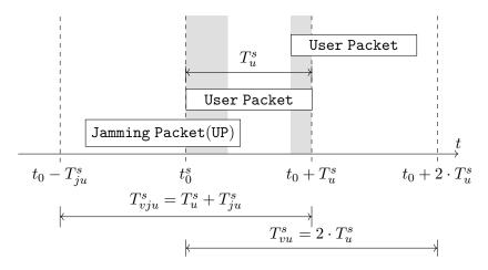
Figure 4.3: Vulnerability periods for an user packet
