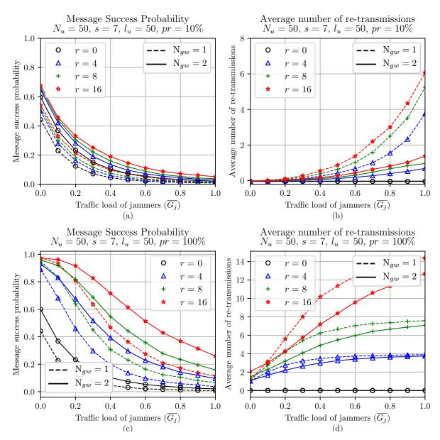
Figure 5.12: Performance evaluation of a LoRaWAN network with re-transmissions and Gateway diversity under jamming (a) Message Success Probability with pr=10%, (b) Average number of re-transmissions with pr=10%, (c) Message Success Probability with pr=100%, and (d) Average number of re-transmissions with pr=100%
