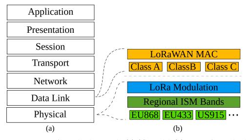
Figure 2.1: LoRaWAN technology stack: (a) OSI model, (b) LoRaWAN Technology
