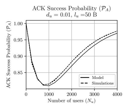
**Figure 4.5:** ACK success probability  $(\mathcal{P}_{\mathcal{A}})$  of a LoRaWAN-like network without jamming
