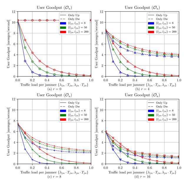
**Figure 5.13:** Performance impact of jammers when varying the jammer strategy: (a) r = 0, (b) r = 4, (c) r = 8 and (d) r = 16
