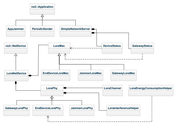
Figure 4.9: UML Schema of the ns-3 LoRaWAN module.
