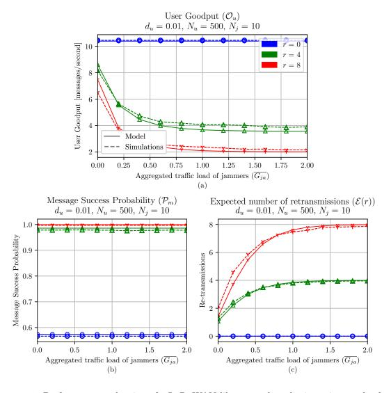
**Figure 5.4:** Performance evaluation of a LoRaWAN-like network under jamming on the downlink channel: (a) User goodput  $(\mathcal{O}_u)$ , (b) Message Success Probability  $(\mathcal{P}_m)$  and (c) Expected number of re-transmissions  $(\mathcal{E}(r))$ .
