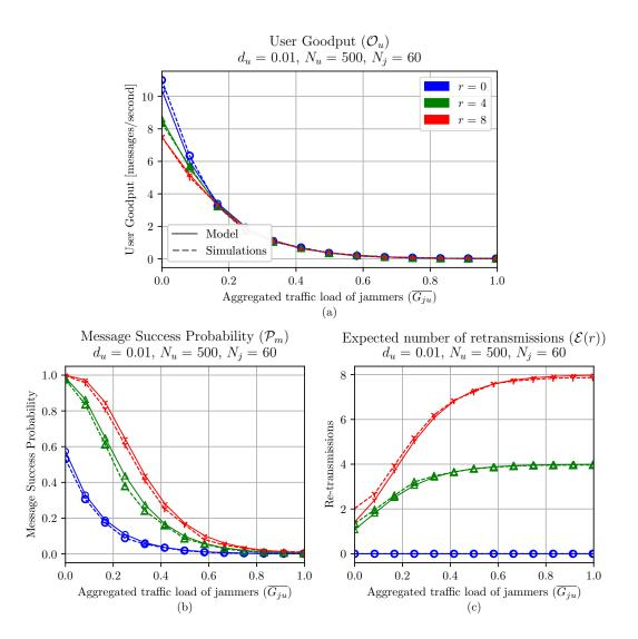
Figure 5.3: Performance evaluation under jamming on the uplink channels: (a) User goodput  $(\mathcal{O}_u)$ , (b) Message Success Probability  $(\mathcal{P}_m)$  and (c) Expected number of re-transmissions  $(\mathcal{E}(r))$ .
