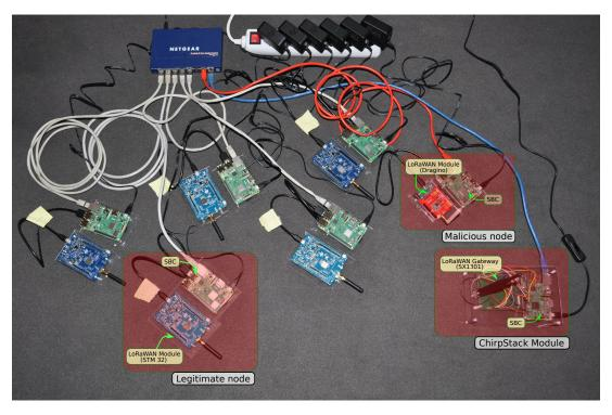
Figure 6.12: LOFRASEA test-bed hardware implementation.
