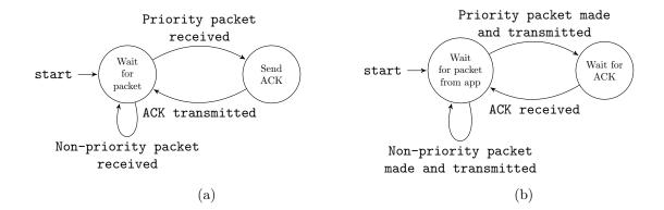
Figure 4.8: Finite state machine for the re-transmissions scheme: (a) NS side, (b) ED side.
