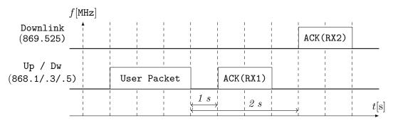
Figure 2.3: LoRaWAN Class A Transmission Schedule
