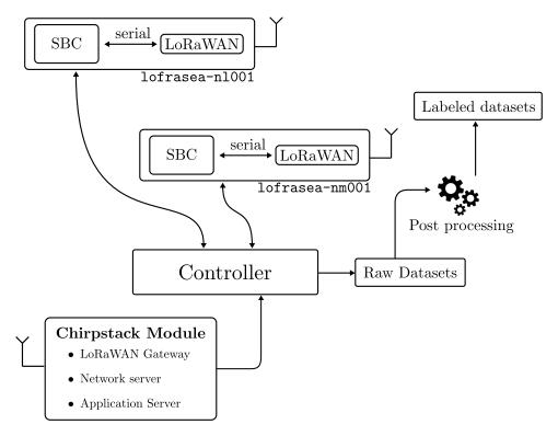
Figure 6.11: Top level architecture of the LOFRASEA test-bed.
