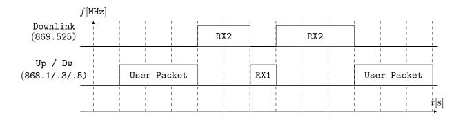
Figure 2.5: LoRaWAN Class C Transmission Schedule
