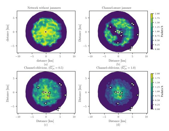
**Figure 5.14:** Throughput per user (packets/h) of a LoRaWAN network under jamming attacks,  $\blacktriangleright$  represents the GW and  $\triangleleft$  represents a jammer.
