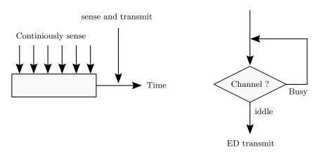
Figure 6.2: Carrier Sense Multiple Access.
