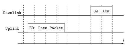
**Figure 4.1:** Packet Scheduling with ACK and user data packets on a different channel but identical SF
