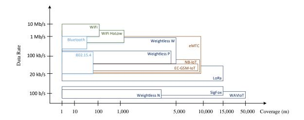
Figure 1.2: Data rate and coverage of IoT wireless technologies.
