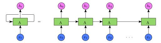
**Figure 6.3:** Top-level diagram of a RNN
