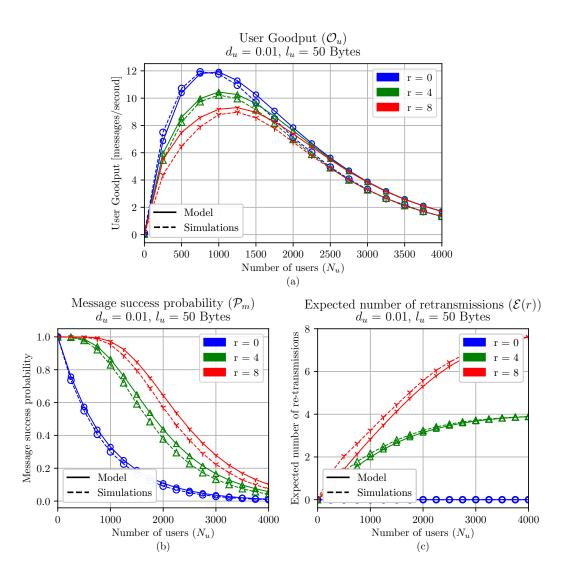
**Figure 5.1:** Performance evaluation without jamming: (a) User goodput  $(\mathcal{O}_u)$ , (b) Message Success Probability  $(\mathcal{P}_m)$  and (c) Expected number of re-transmissions  $(\mathcal{E}(r))$ .
