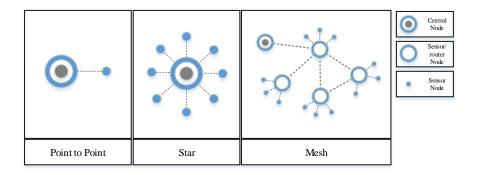
Figure 1.3: IoT Wireless Technologies Topologies.
