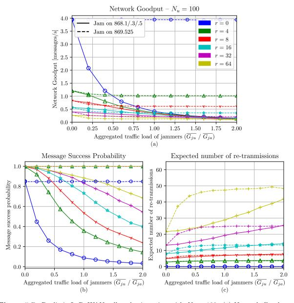
Figure 5.7: Realistic LoRaWAN cell under jamming with  $N_u = 100$ : (a) Network Goodput, (b) Message Success Probability and (c) Average Number of Re-transmissions.
