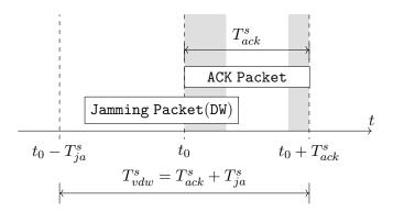
Figure 4.4: Vulnerability period for an ACK packet
