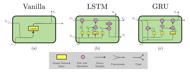
**Figure 6.4:** Different types of RNN: (a) Vanilla, (b) LSTM and (c) GRU. Figure adapted from [159]
