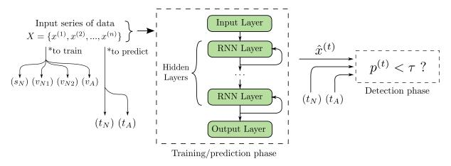
Figure 6.5: RNN jamming detection model
