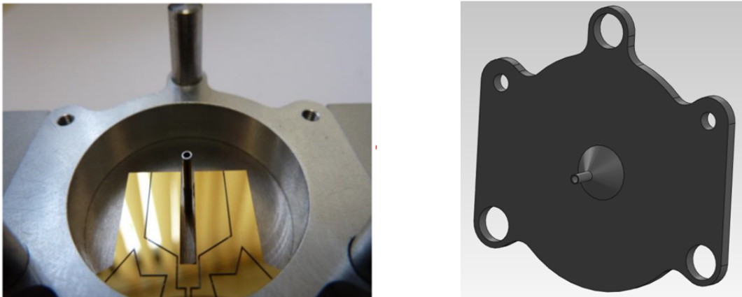
Figure 3.21: Photograph of experimental setup: C2 with acoustic recovery cavity and dual tube resonators (left). CAD view of a designed cavity wall with integrated tube (right).
