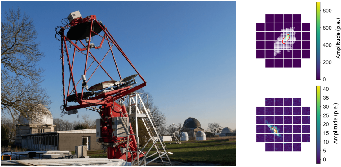
Figure 7.6: Left: The GCT prototype at the Meudon site of the Observatory of Paris. The telescope is equipped with two circular M1 panels out of six. Right: examples of air shower images detected by the CHEC-M camera during the spring 2017 campaign. Credit: Observatoire de Paris. (image source: Dmytriiev et al. (2019b) )
