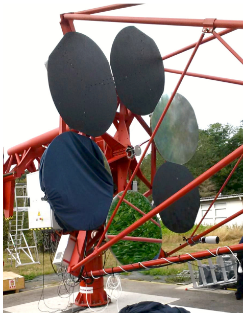
Figure 7.7: A photo showing new M1 segment installed in August 2020 with improved surface polishing (bottom) to be compared with the old M1 element produced in 2014 (top-right). Credit: H. Sol, 2020.
