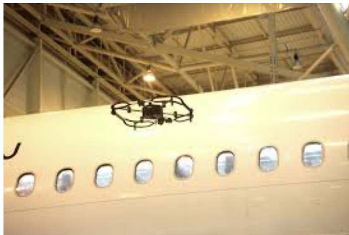
FIGURE 3: Donecle aircraft inspection drone system [54].
