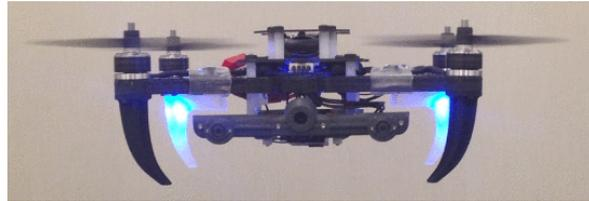
FIGURE 3.8: The smallest drone available on the market that uses VIO to estimate its own position announced by Qualcomm [203]. (Figure captured from [130])
