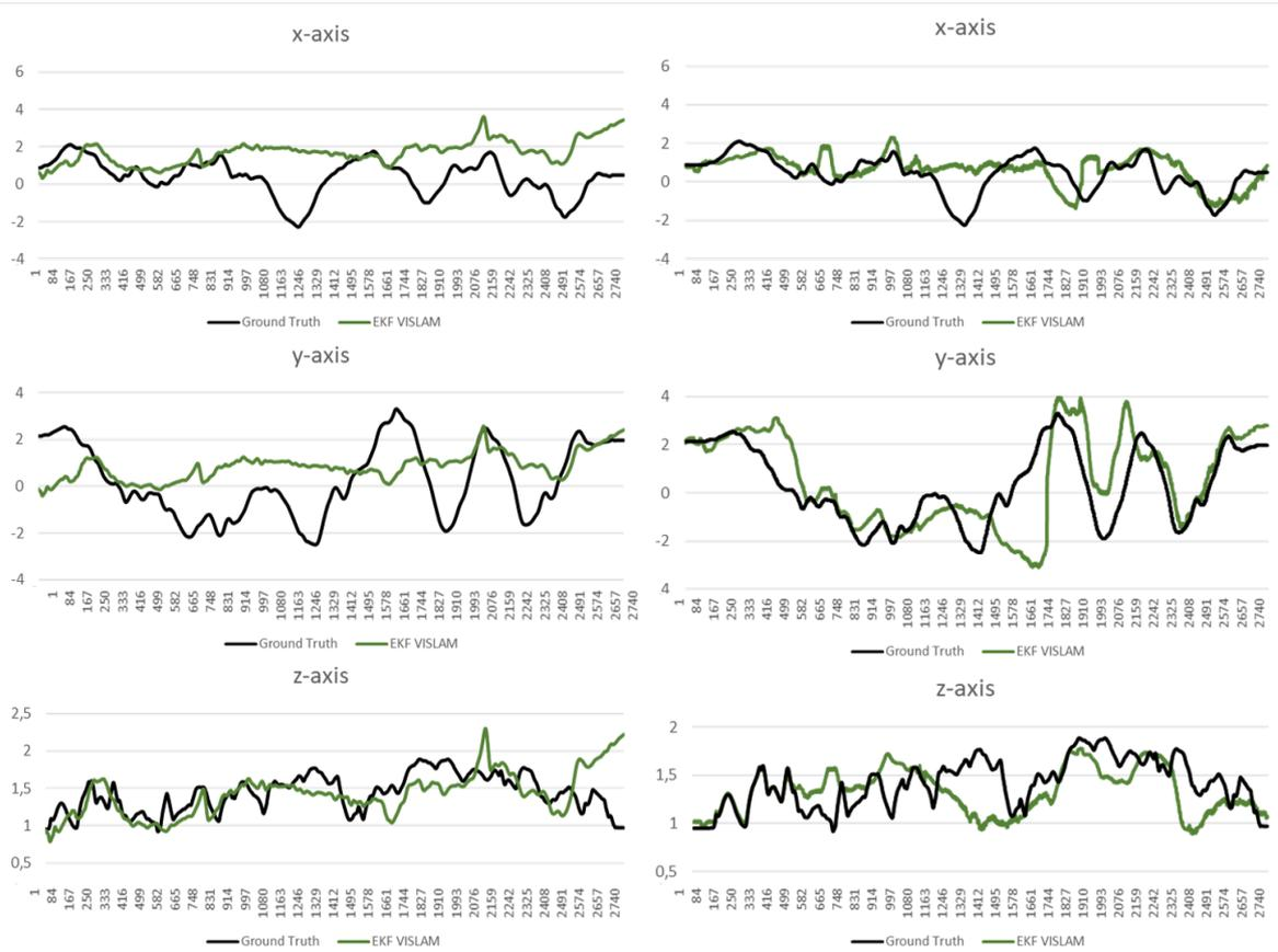
FIGURE 5.6: On the left: EKF VI system without any scale estimation *vs.* EuRoC dataset (V101) ground truth; On the right: EKF VI system with scale estimation, based on the IMU pose computed between two images, *vs.* EuRoC dataset (V101) ground truth ( $m$ ) (horizontal axis shows the IDs of the processed frames)
