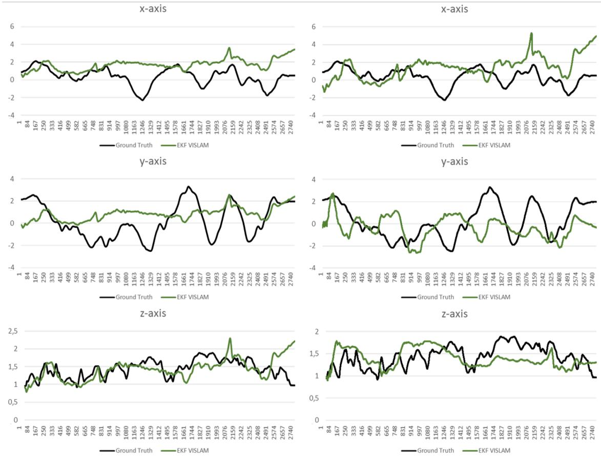
FIGURE 5.7: On the left: EKF VI system without any scale estimation *vs.* EuRoC dataset (V101) ground truth; on the right: EKF VI system with scale estimation, based on the rate between inertial and fused poses, *vs.* EuRoC dataset (V101) ground truth ( $m$ )
