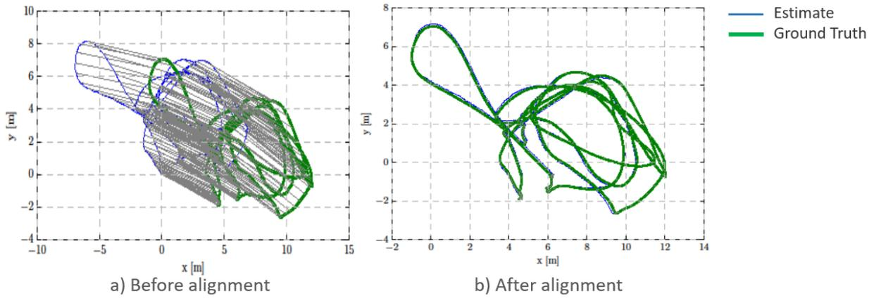
FIGURE 5.19: Context Adaptive VI Tracking (before and after alignment) vs. EuRoC dataset (MH03) ground truth ( $m$ ) (gray lines represent the states correspondences with a step of ten poses)
