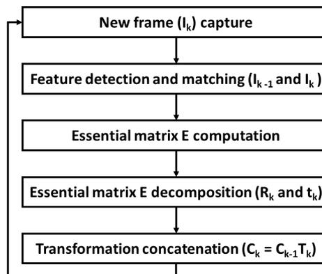
FIGURE 1.14: An overview of the 2D-to-2D algorithm [190]
