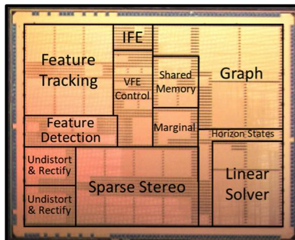
FIGURE 3.12: Photo of Navion chip (die) [203]
