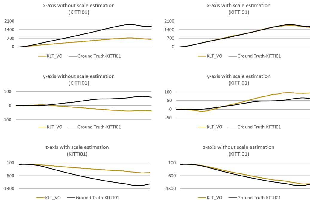
FIGURE 5.4: KLT-based Visual Odometry (with and without scale) vs. KITTI 01 ground truth trajectories ( m )
