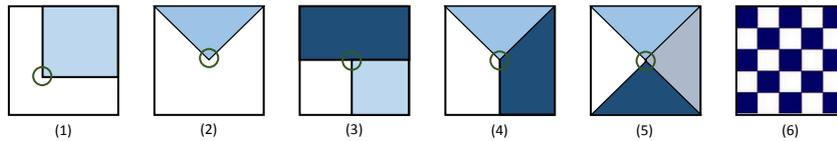
FIGURE 1.7: Several classical types of classical points of interest. (1) L junction, (2) V junction, (3) T junction, (4) Y junction, (5) X junction and (6) point of strong texture variations (checkerboard junction)
