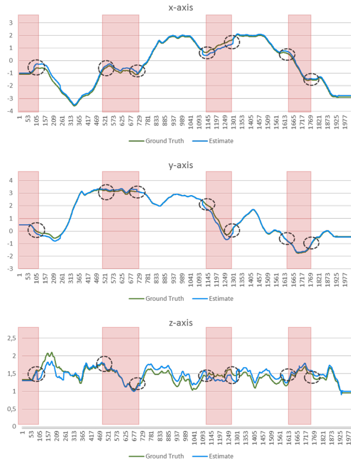
FIGURE 5.21: Context Adaptive VI Tracking vs EuRoC dataset ground truth (V201)( m ). The circles mark the switching areas between the two modes: the KLT-ORB method and the EKF VI method. The red rectangles denote the trajectory parts that are from the KLT-ORB method. The others are the trajectory parts that are from EKF VI method (horizontal axis shows the IDs of the processed frames)
