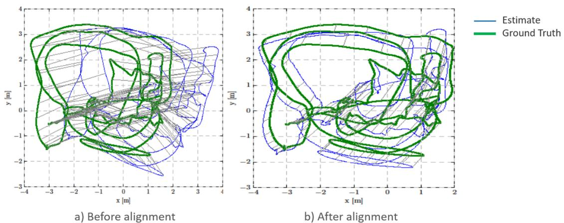
FIGURE 5.16: EKF VI tracking odometry (aligned trajectory) *vs.* EuRoC dataset (V203) ground truth ( $m$ ) (gray lines represent the states correspondences with a step of ten poses)
