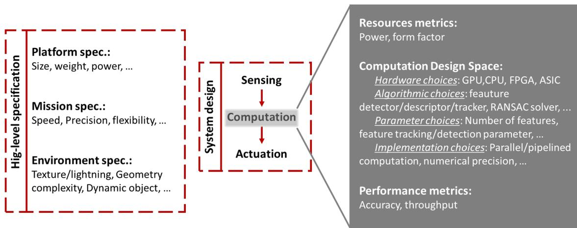
FIGURE 3.9: Co-design method overview (algorithm-hardware trade-off) (inspired from [232])
