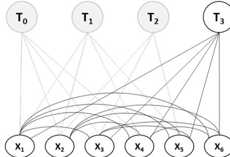
FIGURE 1.6: Filtering-based approach (T: camera pose, X: feature/landmark)
