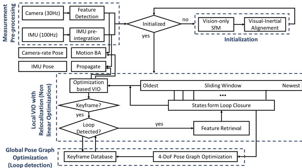
FIGURE 2.10: VINS Mono System framework, reproduced from [175]
