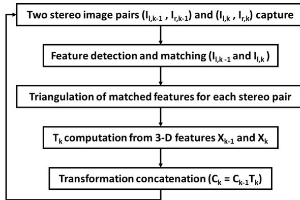
FIGURE 1.16: An overview of the 3D-to-3D algorithm [190]
