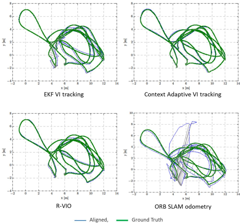
FIGURE 5.23: Trajectories comparison of different systems (ORB SLAM (Odometry), R-VIO, EKF VI tracking and the proposed system: Context Adaptive VI Tracking) on an easy-medium EuRoC dataset (MH03) ( $m$ ) (gray lines represent the states correspondences with a step of ten poses)
