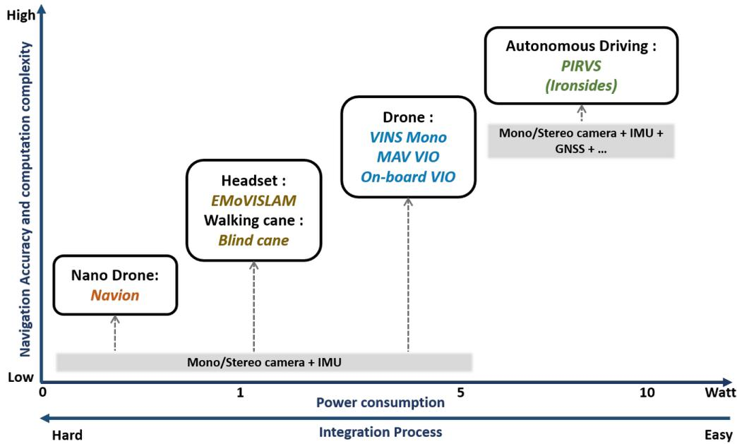
FIGURE 3.17: A classification of embedded tracking systems
