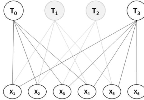
FIGURE 1.5: Optimization/Keyframe-based approach (T: camera pose, X: feature/landmark)
