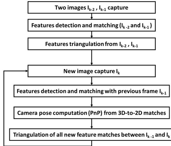
FIGURE 1.17: An overview of the 3D-to-2D algorithm [190]
