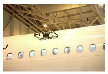
FIGURE 3: Donecle aircraft inspection drone system [54].
