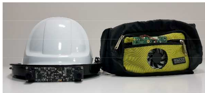
FIGURE 3.14: Wearable EMOVI-SLAM (a head-gear and a processing unit tied on waist) (from [211])
