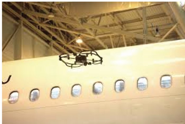
FIGURE 3: Donecle aircraft inspection drone system [54].
