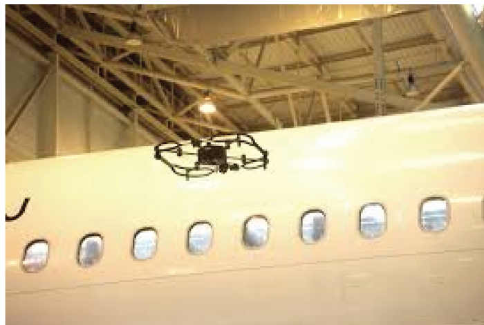
FIGURE 3: Donecle aircraft inspection drone system [54].
