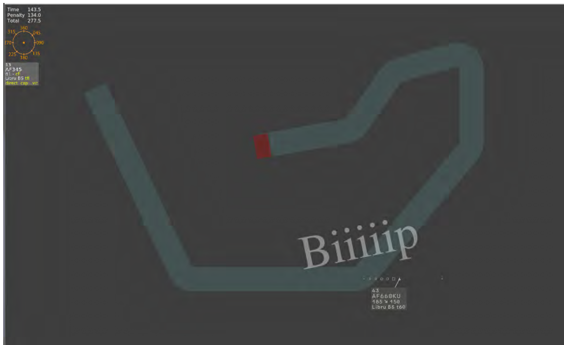
Figure 2. A scenario with one aircraft. The top left corner displays a compass rose to help participants choose the aircraft flight path. On the bottom right a visual alert was displayed due to an aircraft leaving the flight path.
