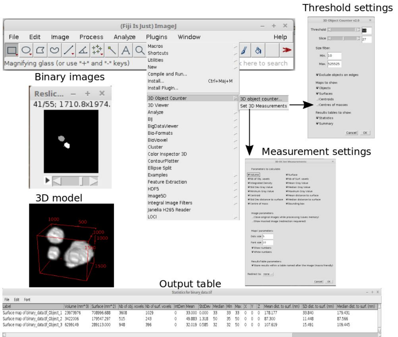
Figure 2.31 – 3D Object Counter plugin from Fiji provides all geometric topology information of detected objects in the cluster.
