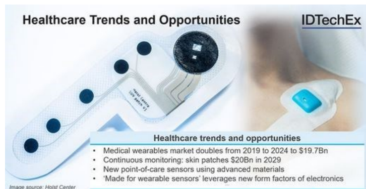
Figure 1. 6 Shows an electronic skin patch - an integration of flexible and printed electronics with conventional electronics to create a wearable patch. Holst Centre predicts healthcare trends and opportunities growing doubling from 2019 to 2024 3 .
