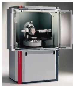
Figure B. 2 Bruker's X-ray Diffraction D8-Discover instrument
