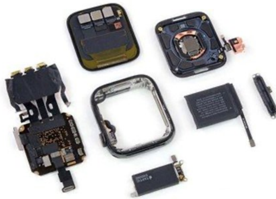
Figure 1. 3 Teardown of an Apple Watch © Serie 5 showing the complex packaging of Printed Circuit Boards, electronic modules and battery interconnected through flexible connectors. Source: iFixit.com
