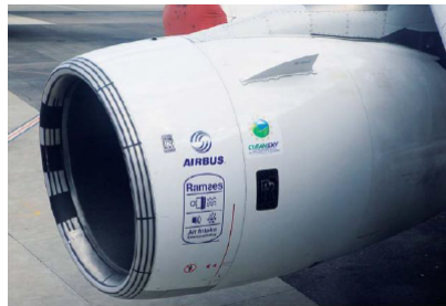
Figure 2.3: Installation of an acoustic liner at the intake of turbofan engine [53].
