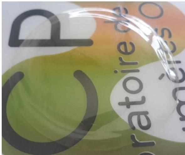
Figure III.15: Picture of a chitosan film (Ch. 78 10 g/L and AA 10 mL/L).
