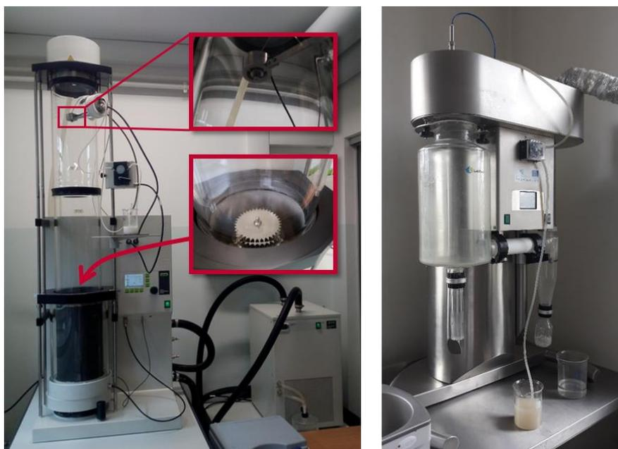
Figure II.4: Spray-dryer from Büchi (left), with a zoom on the head and on collecting electrodes. Spray-dryer from Lab-Plant (right).
