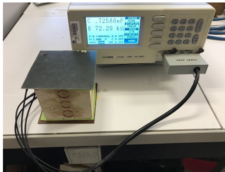
Figure 2.14: Experiential setup for the measurement of resistivity by LCR
