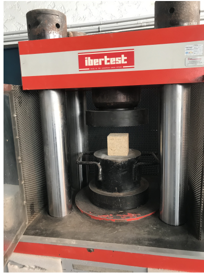
Figure 2.8: Experimental setup for compression test
