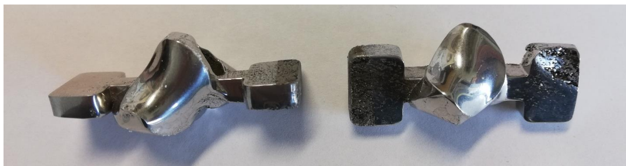
Figure 5: Mirror-like implant processed by SLM and superfinished
