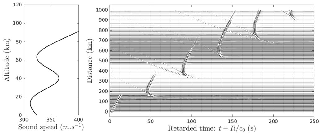
FIGURE 2.2 : Propagation of an impulsive signal in an atmosphere characterised by the sound speed profile given on the left. Time scale has been translated using a reference sound speed  $c_0 = 330 \text{ m.s}^{-1}$ . The source signal has a central frequency at 0.4Hz.
