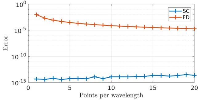
FIGURE 2.6 : Error of the computation of the spectrum in the case of a finite differences scheme (FD) and a spectral collocation approach (SC) for different number of points per wavelength.
