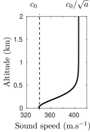
FIGURE 2.5 : Celerity profile of the boundary profile defined in (2.59).  $c_0$  stands for the celerity at the ground,  $a$  sets the celerity for high altitudes and  $H$  the height of the boundary layer. Here,  $c_0 = 340\text{m.s}^{-1}$ ,  $a = 0.7$  and  $H = 250\text{m}$ .
