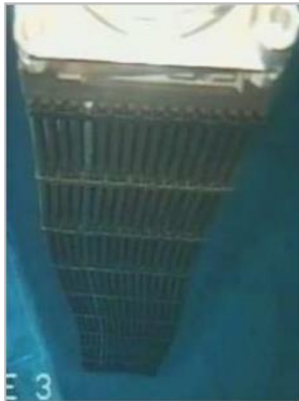
Figure 5-1 - View of a PWR bowed fuel assembly [12]
