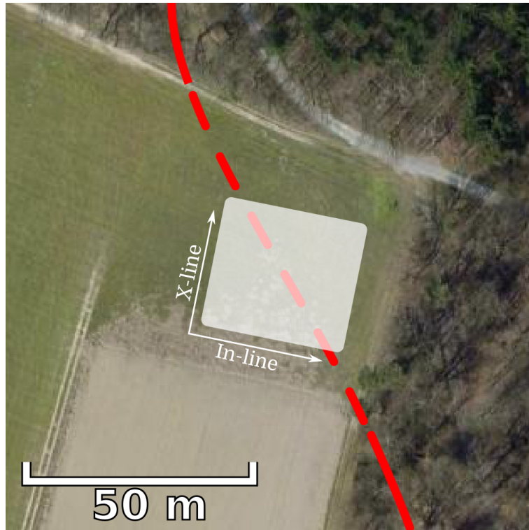
Figure 4.10: Basemap of the seismic data acquisition at Rheinstetten, Germany. The solid red line represents the existing trench line. The dashed red line represents the buried trench. A white box draws the area of the seismic acquisition.
