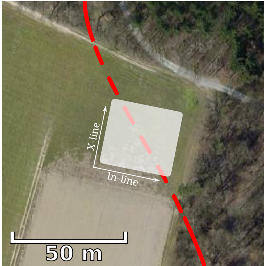
Figure 3.1: Basemap of the acquisition at Rheinstetten. Red solid line represents the existing location of the trench, red dashed line represents the possible buried location of the trench line, and the white rectangle represents seismic acquisition location.
