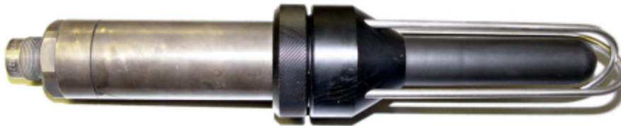
Figure 8: A sample of hydrophone, a pressure sensitive seismic recorder device. It is usually used in marine environment (Wikipedia contributors, 2020a).
