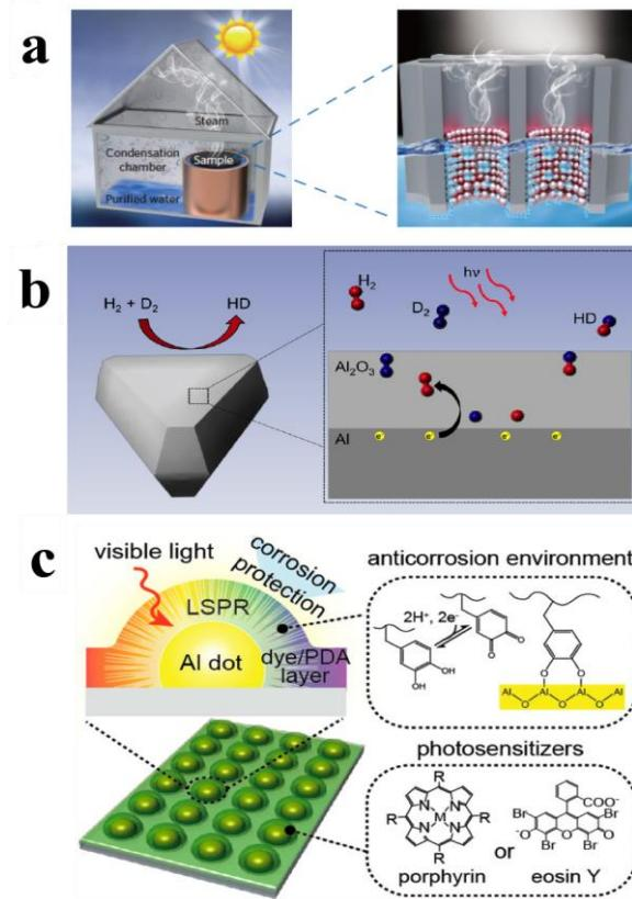
**Figure 1.10.** (a) Experimental setup for solar desalination.<sup>63</sup> (b) Scheme of hydrogen dissociation using Al nanocrystals.<sup>22</sup> (c) Scheme of Al nanoarrays for plasmonic-enhanced light harvesting.<sup>65</sup>
