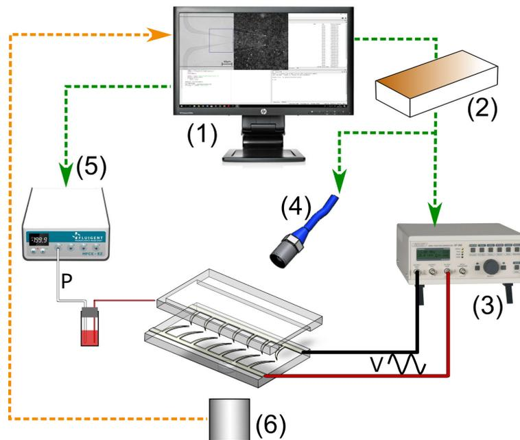
**Figure. 4.1** Experimental set-up for dielectrophoresis measurements in microfluidic systems. (1) PC workstation for global control of experiment and recording of video-microscopy. (2) Arduino single board controller. (3) Electronic function generator used to polarise electrodes. (4) High-power LED coupled into fibre and focused inside the microchannel. (5) Fluigent pressure controller. (6) Optical microscope with attached camera and spectrometer.
