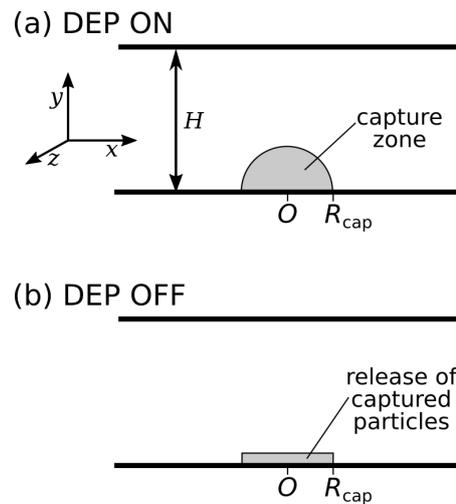
**Figure. 5.21** Schematic of the geometry of the system used in numerical modelling (cross-section in the  $xy$  plane at  $z = 0$ ). (a) Hemisphere where the particles have a non-zero probability of being capture during the "DEP ON" phase. (b) Initial condition for the free diffusion upon entering the "DEP OFF" phase.
