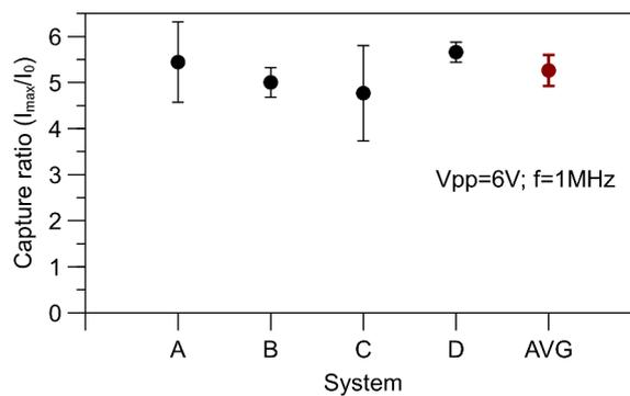
**Figure. 5.18** Capture ratio at  $t = 4$  s of particles release as a function of the device at 6 Vpp and frequency 1 MHz. Data points indicate individual measurements in different devices. Red data point represents the meaning of all points with the standard deviation (95% confidence interval) coming from the experiment measurement.
