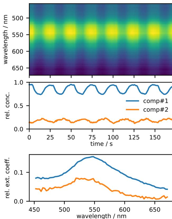
**Figure. 7.4** (*top*) DEP-modulated extinction spectra of an aqueous dispersion of a mixture Au40-LA and Au80-LA (spectrotemporal recording). (*middle*) relative concentration traces for the two principal components reconstructed by target transformation from the singular value decomposition of the spectrotemporal matrix. (*bottom*) The corresponding extinction spectra. The reconstructed concentration traces and extinction spectra reproduce the recorded data.
