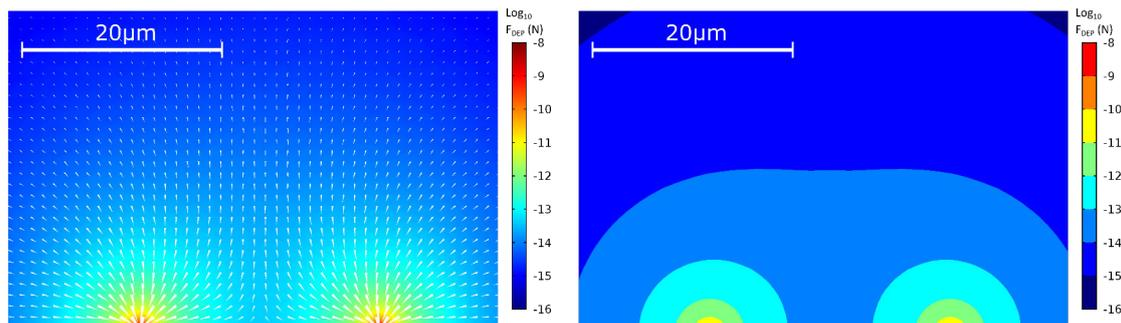
**Figure. 5.17** (*left*) False colour image (side view) of decadic logarithm of the magnitude of the dielectrophoresis force near the electrode tips. The direction of the force is represented with arrows. (*right*) Threshold false colour image with decadic logarithm of DEP forces clarifying the radical dependence of the force around the electrode tips.
