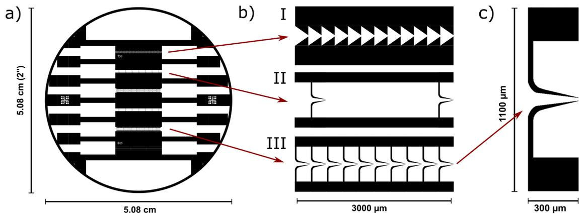
**Figure. 4.2** a) Architecture (and lithography mask) of the hook electrodes chosen for the electromicrofluidic device. b) I- Christmas tree row of electrodes. II- Hook row of electrodes spaced by  $1400 \mu\text{m}$  between each pair. III- Hook row of electrodes without spacing between each pair. c) Building brick of the micro puce
