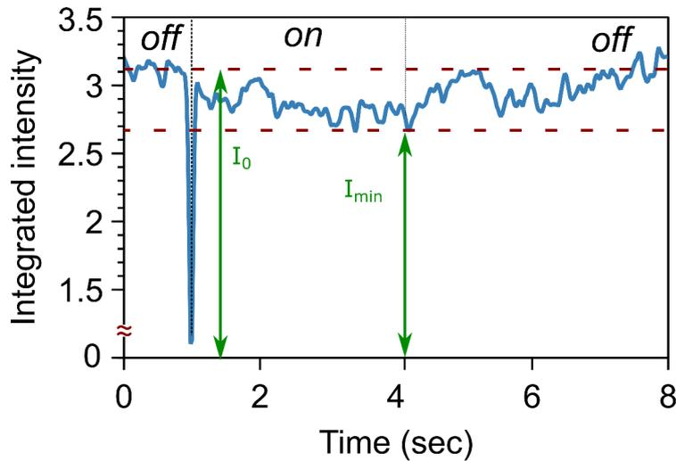
**Figure. 5.13** Integrated intensity as a function of time in the monitored area of dielectrophoretic capture of 200 nm latex nanospheres applying an electric field amplitude of 7 V<sub>pp</sub> and a frequency of 6 MHz using fluorescence videomicroscopy (50 fps). The signal was averaged 25 "ON-OFF" cycles.
