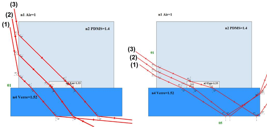
**Figure. 4.20** (*left*) Examples of bad angles for light injection in the system used in this work leading to high background noise. (*right*) Best angles to avoid stray light from reflections in the microfluidic system.
