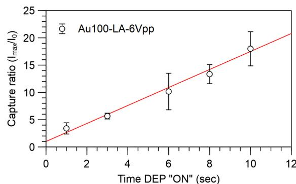
**Figure. 5.10** Capture ratio as a function of the electric field time applied. For each cycle, a time of 5 seconds was fixed to let particles diffused freely. The red line corresponds to the fit of experimental dots.
