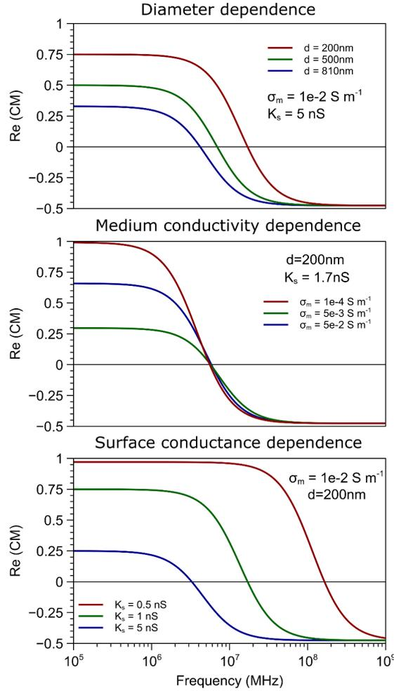
**Figure. 5.11** (top) Theoretically calculated CMF as a function of the diameter of the particles ( $d$ ), with  $\sigma_m = 1.10^{-2} \text{ S m}^{-1}$  and  $K_s = 5 \text{ nS}$ . (middle) CMF as a function of the conductivity of the medium ( $\sigma_m$ ), with  $d = 200 \text{ nm}$  and  $K_s = 1.7 \text{ nS}$ . (bottom) CMF as a function of the particle surface conductance ( $K_s$ ), with  $d = 200 \text{ nm}$  and  $\sigma_m = 1.10^{-2} \text{ S m}^{-1}$ .
