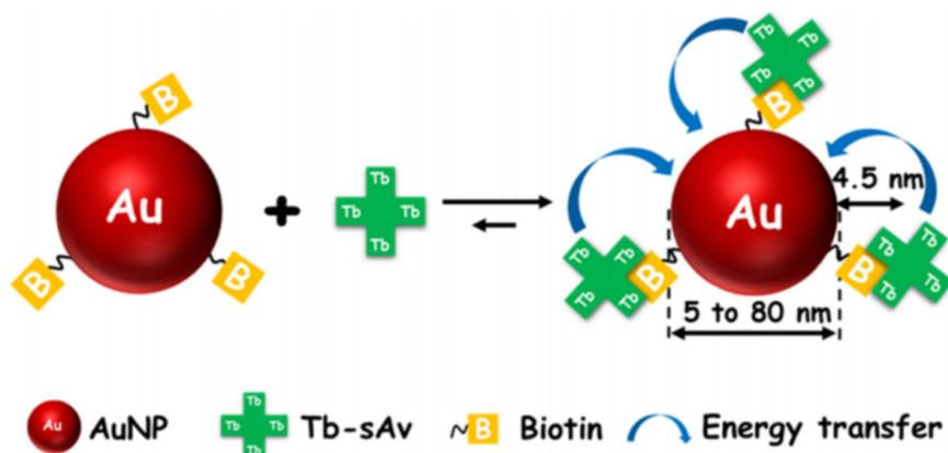
**Figure. 7.1** Schematic representation (not to scale) of the assemblies of Tb-labeled sAv (Tb-sAv) and biotinylated AuNPs (biot-AuNPs), wherein excitation energy transfer occurs. A distance of 4.5 nm was estimated using a radius of 3 nm for sAv plus 1.5 nm for the biotin and linker attached to the AuNP.
