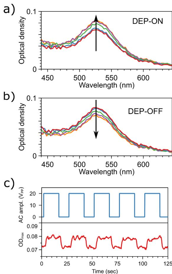
**Figure. 6.5** DEP-modulated optical extinction spectroscopy of Au40-LA in aqueous solution. (a) Evolution of the extinction spectrum in the observation volume during the "DEP ON" phase. (b) Evolution of the extinction spectrum in the observation volume during the "DEP OFF" phase. (c) Amplitude of the applied AC potential (*top*) and evolution of the measured optical density at  $\lambda_{\max} = 526$  nm as a function of time.
