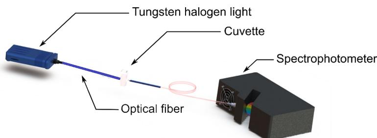
**Figure. 3.2** Set-up used to record extinction spectra
