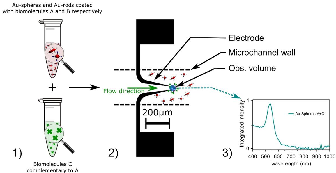
**Figure. 7.5** (1) Schematic representation (not to scale) of the assemblies of AuNPs functionalised with biomolecules A and biomolecules B complementary to A. (2) Schematic top-view of the microfluidic channel and the capture area analysed by the spectrophotometer. Shows the selectivity of the capture as a function of the electric field parameters and affinities of particles coated with biomolecules (3) Extinction spectra of Au-Spheres-A+C capture using dielectrophoresis.
