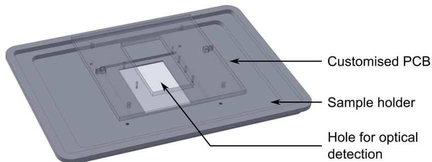
**Figure. 4.11** Sample holder for mounting the electromicrofluidic device on the microscope, including the placement for electrical and optical system
