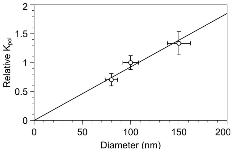
**Figure. 5.24** Relative dielectrophoretic susceptibility  $K_{pol}$  as a function of gold nanoparticle diameter (circles). The  $K_{pol}$  values are relative to the value of 100 nm particles. The solid line suggests a linear relation between  $K_{pol}$  and nanoparticle diameter.
