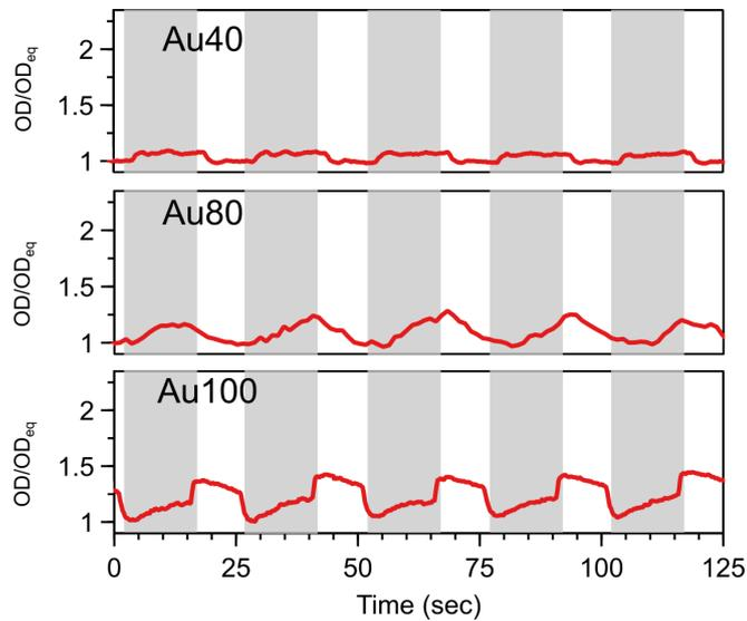
**Figure. 6.6** Selected DEP modulation cycles of Au40-LA, Au80-LA and Au100-LA, in the absence of flow, monitored as the optical density at the wavelengths of the plasmon maximum,  $\lambda_{max} = 526$  nm,  $\lambda_{max} = 549$  nm,  $\lambda_{max} = 572$  nm. The grey areas in the background indicate when the DEP field was active.
