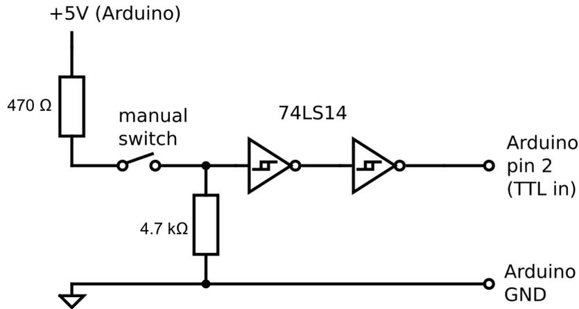
**Figure. 4.24** Electric circuit for interfacing a physical switch to a digital TTL input of the Arduino board.
