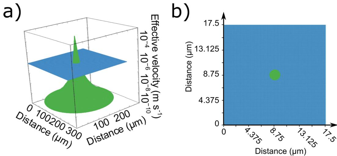
**Figure. 5.2** a) 3D plot of the effective velocity due to DEP ( $\text{m s}^{-1}$ ) for a gold nanoparticle of 100 nm diameter. Dielectrophoresis velocity was plotted for applied voltage 10 Vpp (green). It was compared to the effective velocity due to the DEP and Brownian motion (blue). b) 2D plot of the cross section between both effective velocity. The cross spot has a diameter of  $1.9 \mu\text{m}$ .
