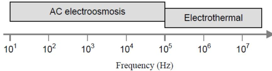
**Figure. 2.13** Frequency ranges in which the different types of electric field-induced fluid flow are observed in AC electrokinetic microsystems. The magnitude of the applied potential was 1 Volt and the separation of the two coplanar electrodes was 25  $\mu\text{m}$ . AC electro-osmosis dominates in the lower frequency range ( $<100$  kHz) and electro-thermal fluid flow at higher frequencies.[105]
