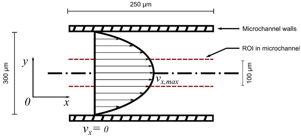
**Figure. 6.8** Representation of the fluid velocity distribution in the microchannel used in this work. Red dotted lines show the region of interest (ROI) selected to analyse the average gold nanoparticles velocity in the microchannel using particles tracking analysis presented in the next part of this section.
