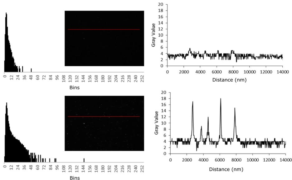
**Figure. 4.22** Comparison of the (*bottom*) new high power white LED illumination to the (*top*) old method using a sample of 100 nm gold nanoparticles deposited on the bottom of a microchannel. (*left*) Histogram of the red line from the image (*right*) Grey value as a function of the distance along the red line on the image.
