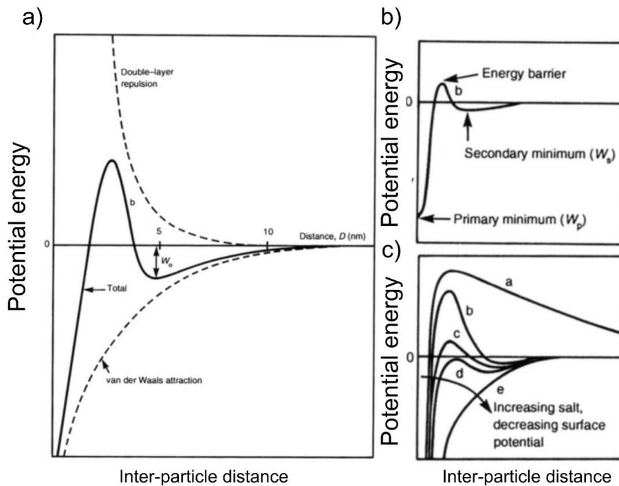
**Figure. 2.9** a) Interaction energy of a system composed of two charged particles in water as a function of the distance between both using the DLVO theory. b) Energy minima and energetic barrier. c) Effect of the ionic strength on the potential curves
