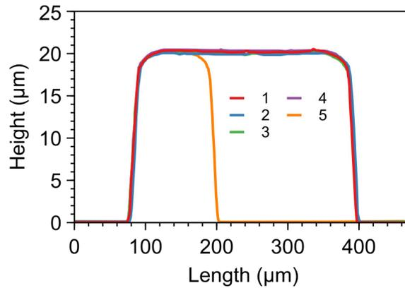
**Figure. 4.8** Thickness of SU-8 deposited by spin coating on silicium wafers. 1 to 4: Profilometric scans of four different molds with a 300  $\mu\text{m}$  width channel. 5: microchannel of 100  $\mu\text{m}$  of width.
