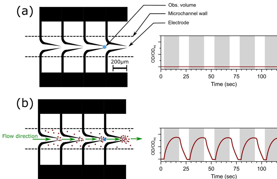
**Figure. 6.4** (a): Schematic top-view of the microfluidic channel showing the relative sizes of electrodes and the capture area (actual diameter = 50  $\mu\text{m}$ ) analysed by the spectrophotometer. (b): Shows the gradual capture of particles along the microchannel. Dashed lines corresponds to microchannel walls.
