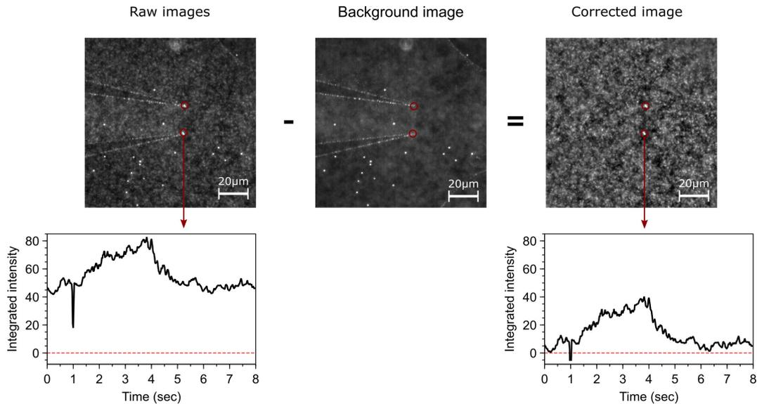
**Figure. 5.4** Top: (*left*) Raw image of 100 nm gold nanoparticles in the microchannel dispersed around electrode tips. (*middle*) One of the background images subtracted from the raw images, removing stuck particles and the signal from PDMS and ITO electrodes scattered light. (*right*) Corrected image (*bottom*) Mean intensity profiles averaged from the red circles before correction and after correction.
