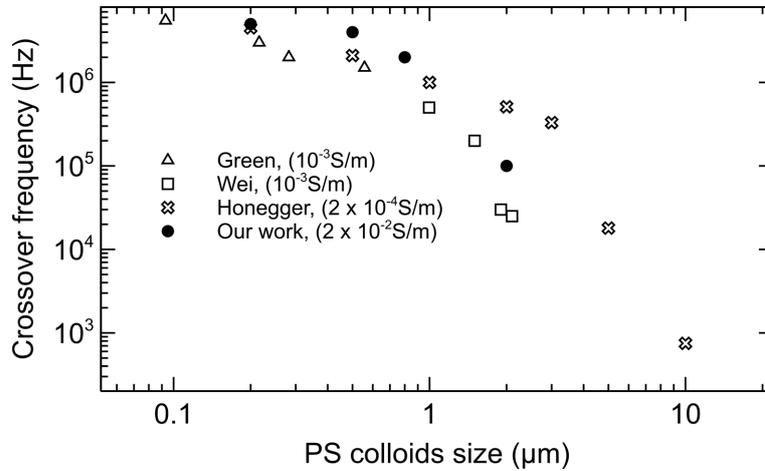
**Figure. 5.14** DEP crossover frequency for polystyrene latex particles: comparison of determination using the capture ratio in microfluidic system carried out in the study, and values from the literature. Capture ratios were measured for all polystyrene latex particles, except particles of 2  $\mu\text{m}$  diameter which were analysed only by direct visual inspection of DEP-induced particle motion.
