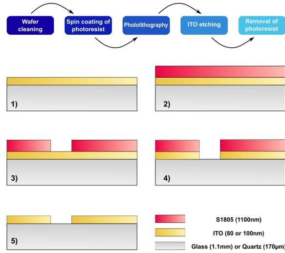
**Figure. 4.3** Steps of the ITO electrodes microfabrication. (1) original state, (2) resin photosensible deposited on, (3) non-exposed resin light removed, (4) etching of ITO, (5) electrodes ready for use
