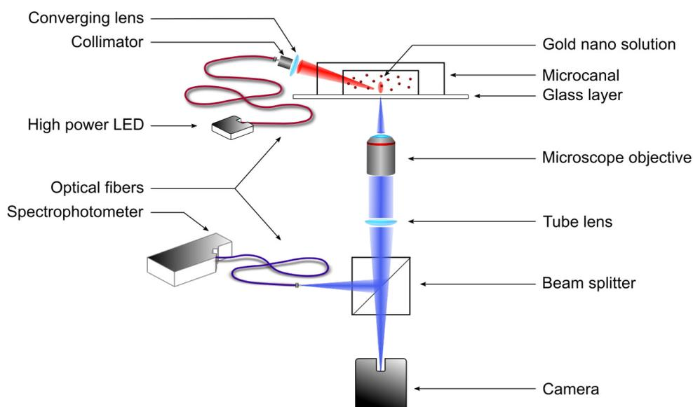
**Figure. 4.14** Scheme of the microscope optical path of the high power LED light source of the colloidal solution samples, and the light emitted by the samples to both detectors, the spectrophotometer and the camera. This setting recorded dark field video-microscopy or scattered light emitted.
