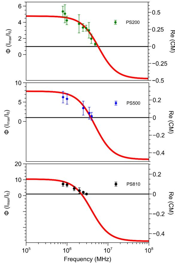
**Figure. 5.12** Experimental capture ratios for polystyrene particles (200, 500, 810 nm) as a function of the frequency at 7 Vpp to determine the crossover frequency. Red lines correspond to model calculations of the Clausius-Mossotti factor, using  $\epsilon_m = 78.5\epsilon_0$ ,  $\sigma_m = 1 \times 10^{-2} \text{ S m}^{-1}$ , and  $K_s = 1.7 \text{ nS}$  (PS200),  $K_s = 2.8 \text{ nS}$  (PS500),  $K_s = 3.1 \text{ nS}$  (PS810).
