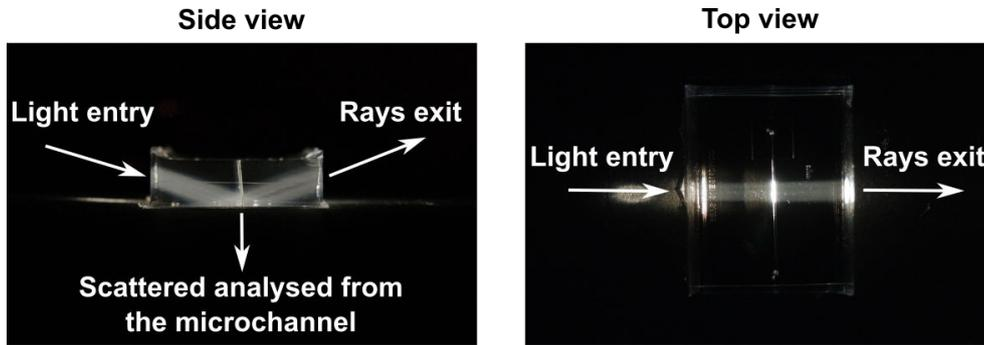
**Figure. 4.21** Pictures coupling light into the PDMS from the side with a  $25^\circ$  incidence angle, using a fibre-coupled LED connected to a collimator and focused with an additional lens. (*left*) Side view (*right*) Top view.
