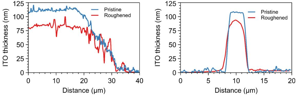
**Figure. 5.8** Analysis of AFM pictures. (*left*) thickness of the ITO along the electrodes. (*right*) thickness of the ITO the electrodes using a cross-sectional profile (perpendicular to the electrode).
