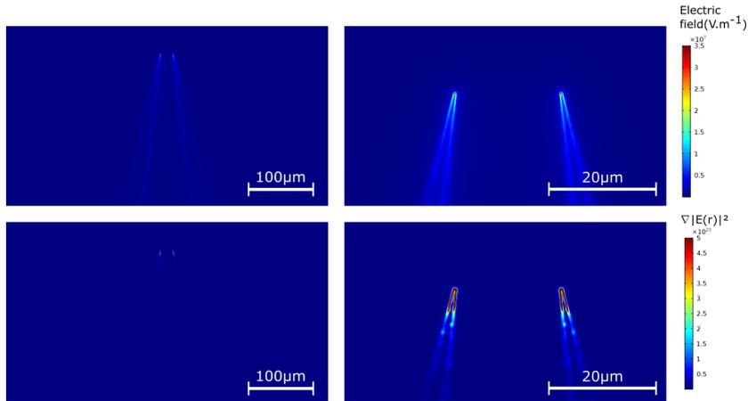
**Figure. 5.15** (*top*) Top view of calculated electrical field strength on electrodes in the microchannel in the electrode plane. (*bottom*) Top view of gradient of the squared norm of the electric field.
