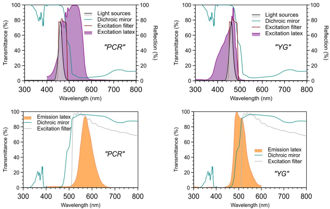
**Figure. 4.16** (top) Spectra of the light source M470-L ( $\lambda_{max} = 470$  nm) superposed on the spectra of the excitation filter (BP420-480), dichroic mirror (DM500) reflection and excitation latex. (bottom) Emission spectra of latex spheres superposed on the spectra of the dichroic mirror (DM500) and the emission filter (BA520IF). (left): Latex with "polychromatic red" (PCR) fluorophores. (right): Latex with "Yellow-Green" (YG) fluorophores.
