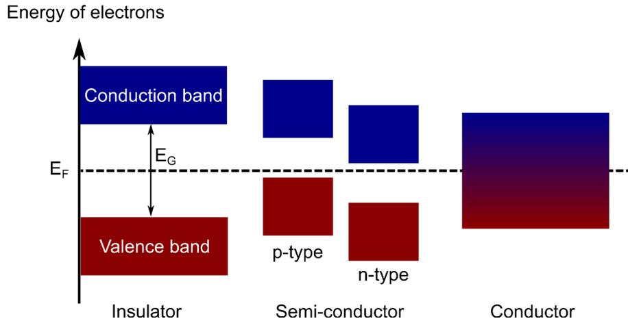
**Figure. 2.5** Schemes of the valence band ( $E_0$ ) and the conduction band for an insulator, semi-conductor and conductor. The Fermi level ( $E_F$ ) is represented with a dotted line, this last is highly dependent on the temperature.  $E_G$  is the band gap energy between the valence band and the conduction band.
