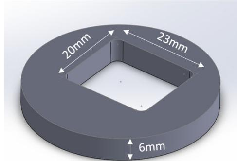
**Figure. 4.9** Plexiglass holder produced using laser cutting to embrace the ideal size of the PDMS slab. It provides PDMS systems with smooth edges that allow for clean injection of the light from the side of the slab
