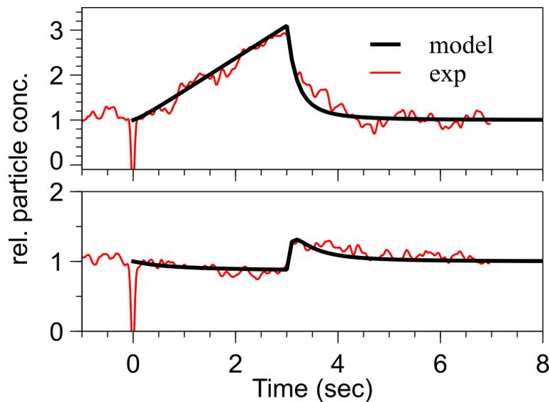
**Figure. 5.23** Time evolution of the particle concentration. Comparison of model (black) and experimental capture curves (red). Capture of 100 nm gold nanoparticles in water at 298 K on the tip of electrode (*top*) and depletion in a ring just outside the capture zone (*bottom*). Experiment: amplitude 5 Vpp, theory: capture rate  $0.8 \text{ s}^{-1}$ .
