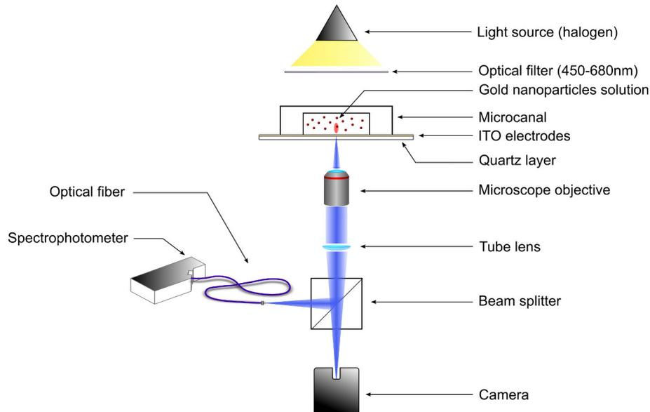
**Figure. 6.1** Schematic of the dielectrophoresis system composed of ITO electrodes, PDMS microchannel and halogen light source, and split detection channel consisting of digital camera and fibre-coupled spectrometer.
