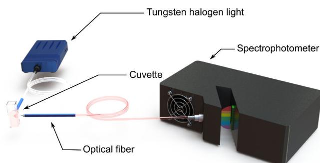
**Figure. 3.3** Schematic representation of the resonant light scattering set up using optical fibres to guide. Scattered light is collected at a fix angle ( $90^\circ$ ) and analysed using a CCD spectrograph
