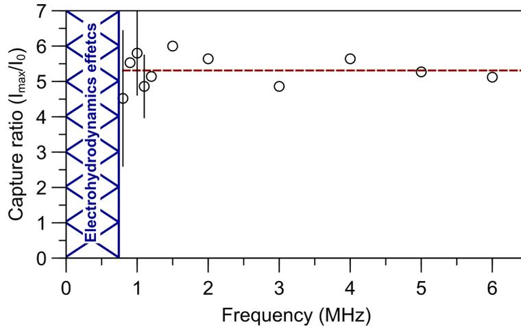
**Figure. 5.19** Capture ratio at  $t = 4$  s of Au100-LA as a function of electric field frequency applying an AC electric potential with amplitude 6 Vpp. The data points indicate the average of individual measurements with the standard deviation (95% confidence interval). The dotted line is the mean value of all measured capture ratios. Frequencies smaller than 800 kHz were not studied due to the appearance of electrohydrodynamic effects that perturb characterization.
