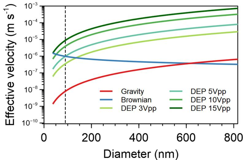
**Figure. 5.1** Effective velocity ( $\text{m s}^{-1}$ ) as a function of the particle diameter. The magnitude of the velocity due to DEP is plotted for voltage applied between 3 to 15 Vpp and compared to the magnitude of the velocity due to the gravity and Brownian motion.
