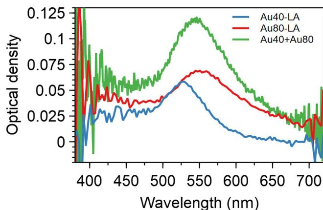
**Figure. 6.11** Spectra of stock solutions Au40-LA, Au80-LA and Au40-Au80 recorded inside the microchannel for an exposure time of 250 ms.
