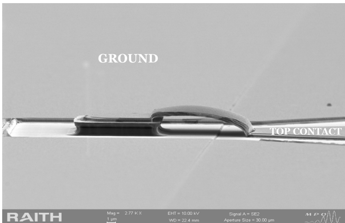
FIGURE 3.18: SEM image of the QCD at 10\ \mu\text{m} mesa size with the air-bridge and the gold coplanar waveguide.
