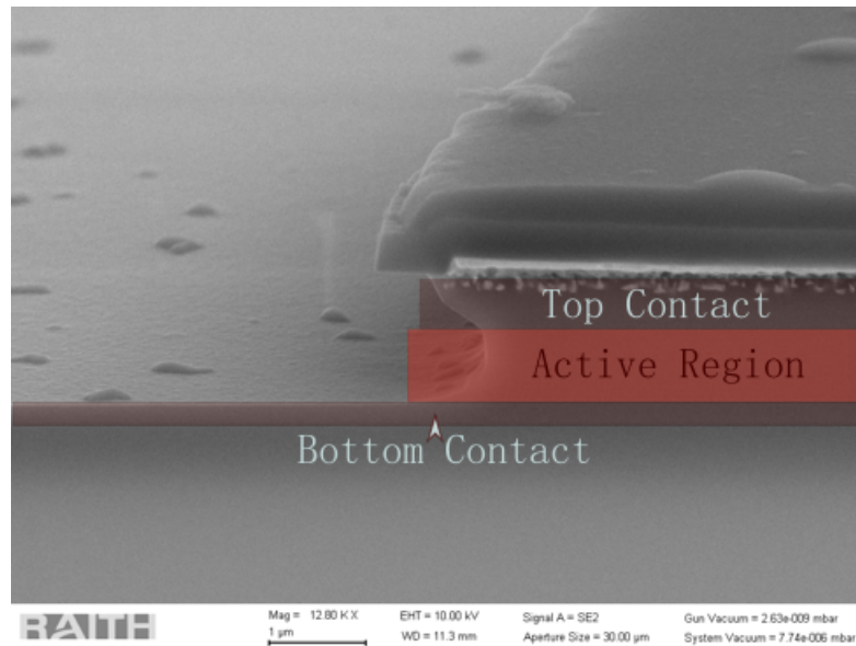
FIGURE 2.13: SEM image of the QCD after wet etching with H_3PO_4 : H_2O_2 : H_2O .
