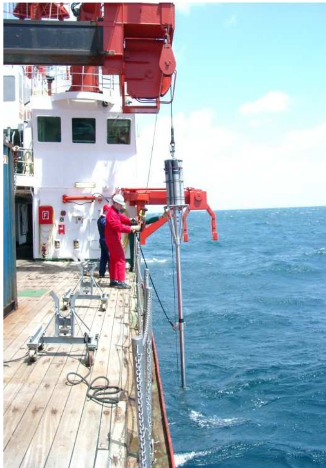
Figure 1.20: The 5.4 m long heatflow measuring probe used in the LITHOS 2017 experiment (Credit: Prof. Heiner Villinger ). The probe is being lowered from the ship deck to the seafloor through a winch cable. The vertical temperature gradient and the thermal conductivity are measured by the probe at each heatflow location.
