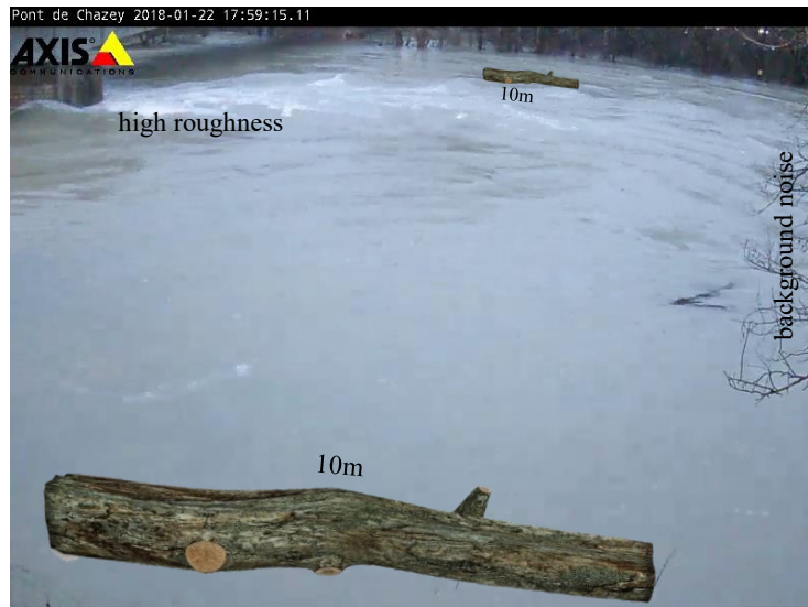
Figure III-13 Wood position can highly affect the quality of detection. Pieces that are passing in front of the camera are detected much better than the pieces far from the camera.
