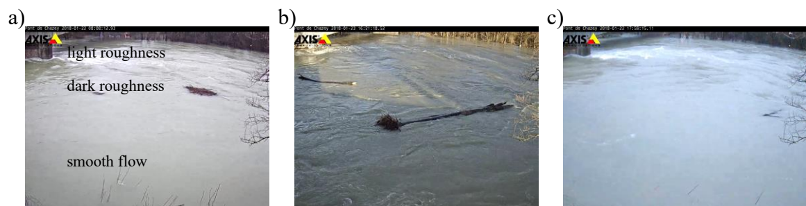
Figure III-12 Different light conditions during (a) morning, (b) noon and (c) late afternoon, results in different frame roughness's and different detection performances.
