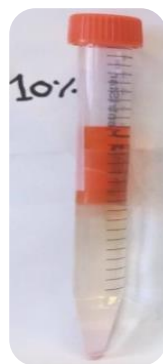
Figure 3: picture of a mixture of 50/50 (v/v) ACN/water and 10 % (m/v) of NaCl salt. Methyl red indicator solution was added and was mainly solubilized in organic phase.
