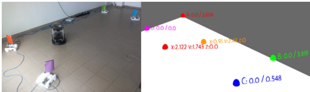
Fig. 14. SecureLoc Platform ( left ), 3D engine overview ( right )
