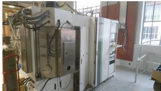
Figure 4.26: Oven for post-annealing of the deposited films after magnetron sputtering.
