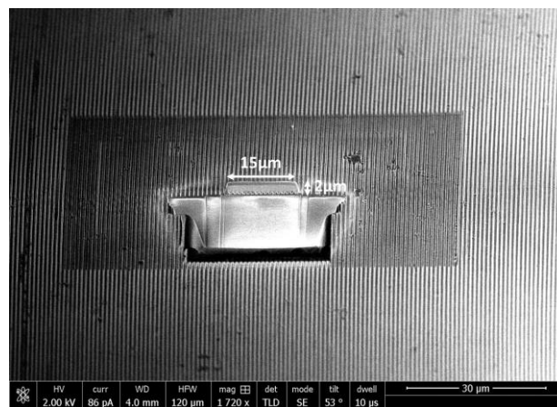
Figure 3.12: Section of the grating area with 15\mu\text{m} \times 2\mu\text{m} .
