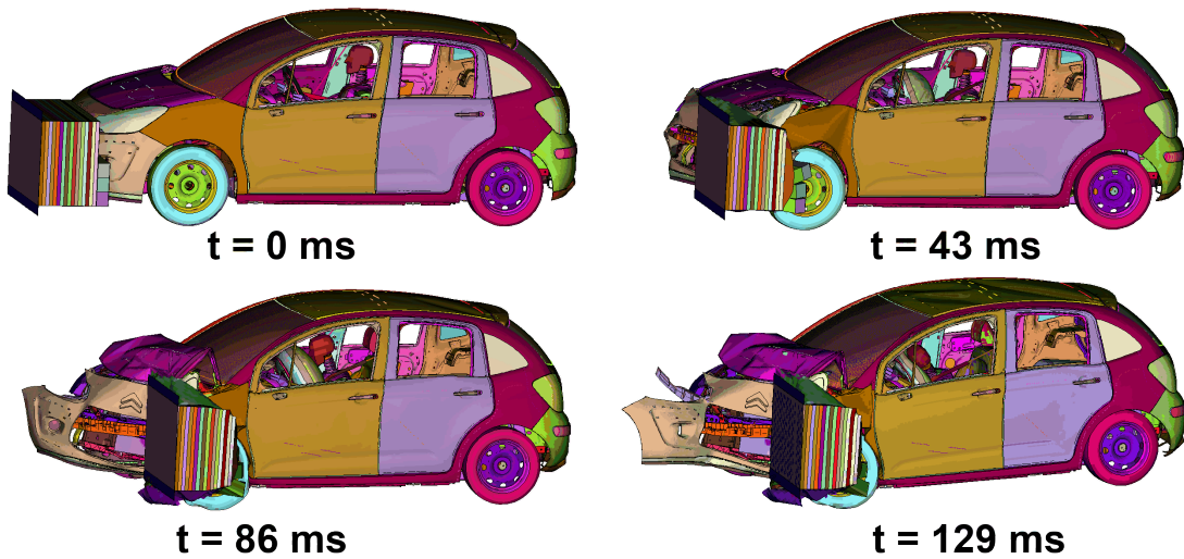
Figure 1.3: Crash simulation example of a frontal offset deformable barrier impact
