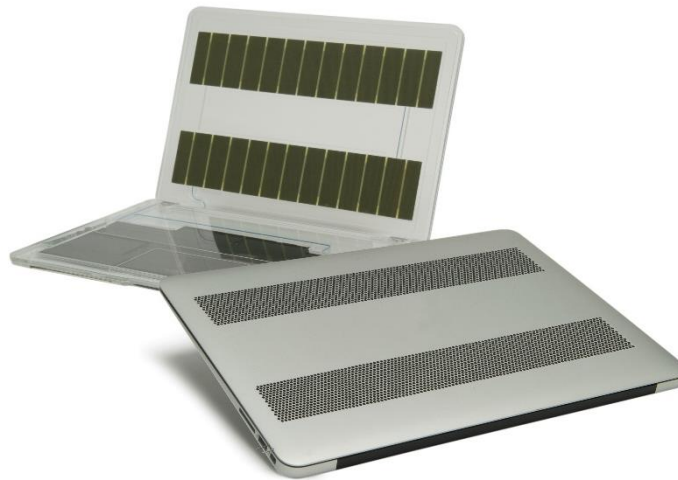
Figure I.10. Prototype of a fuel cell system for powering portable laptop developed by Intelligent Energy.
