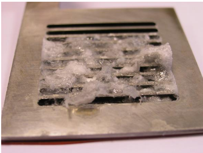
Figure I.13. Photograph of the current collector of an air cathode after prolonged operation in DBFC conditions, highlighting the formation of solid sodium hydroxide. Reprinted from Ref [166].
