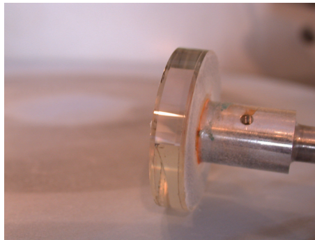
(b) Picture of the stiff arm with the full cylinder being polished to optical quality.
