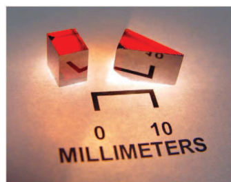
(b) \text{CdSiP}_2 crystal and prism used for refractive index measurements [42]
