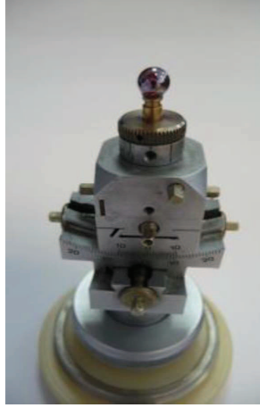
Figure 21: Picture of the 4.99 mm diameter oriented CdSiP 2 sphere, polished to optical quality, used for the phase-matching studies and stuck on a goniometric head.
