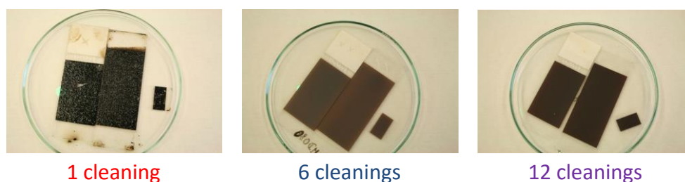
Figure II-46. Visual appearance of coatings after annealing at 300 °C during 30 minutes under argon atmosphere as a function of the number of cleanings N .
