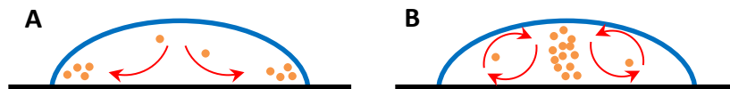
Figure III-33. Scheme of the effect of capillary flux (A) and Marangoni flux (B) on the drying of a droplet on a substrate.
