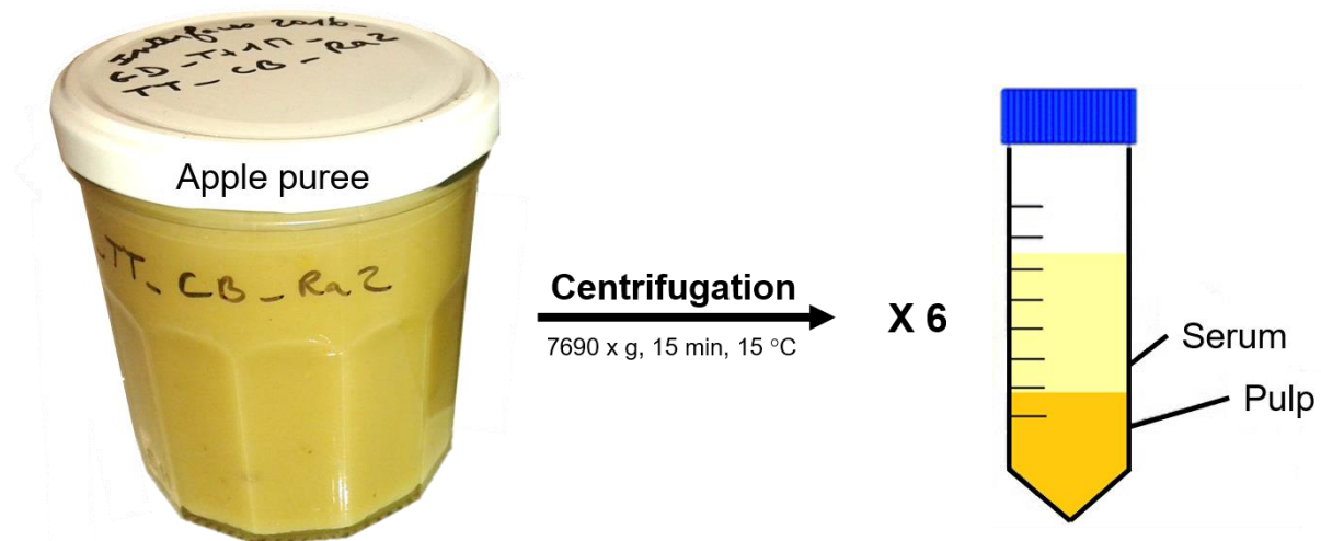
Fig. 49. Separation of apple puree into serum and pulp by centrifugation.
