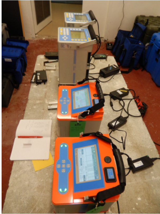
Figure 2.3: Scintrex CG5 and CG6 devices as part of RESIF’s GMob mobile gravimeter facility, in test at the Géosciences Montpellier laboratory (Bertrand, 2019).
