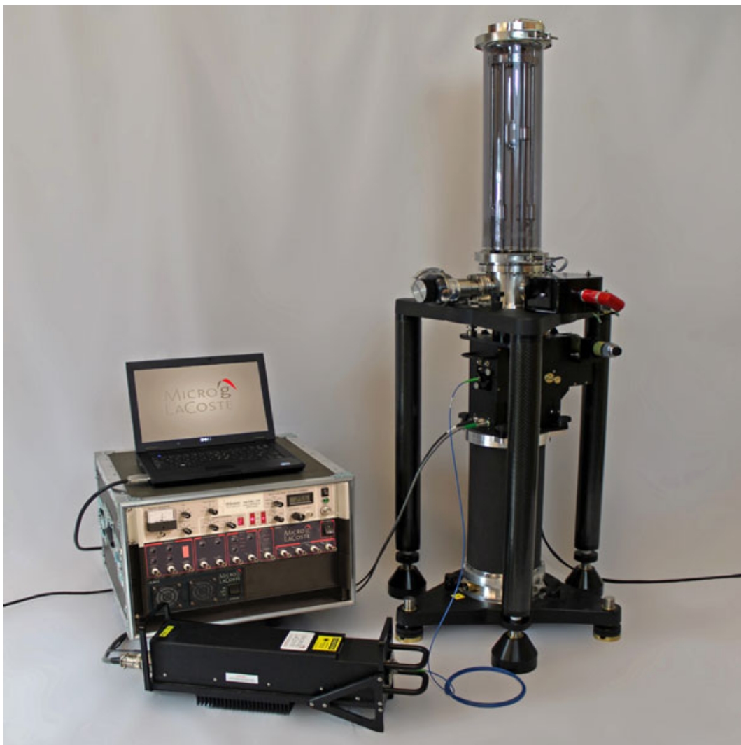
Figure 2.2: FG5-X absolute gravimeter by Micro-g LaCoste Inc., 2020.
