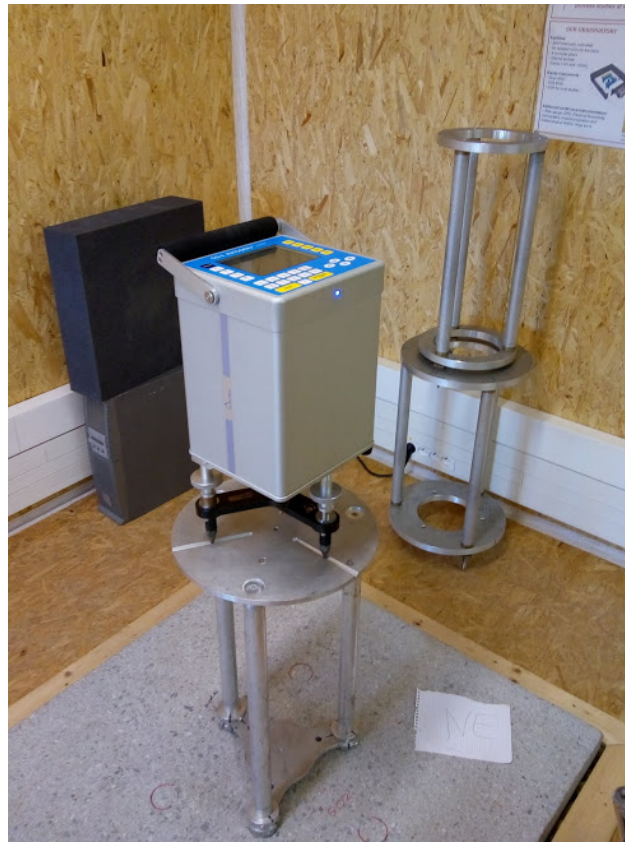
Figure 4.1: Scintrex CG5-1151 relative gravimeter on pillar p_2 on height h_1 in the Larzac observatory in 2018. Photo: Cooke, 2018.
