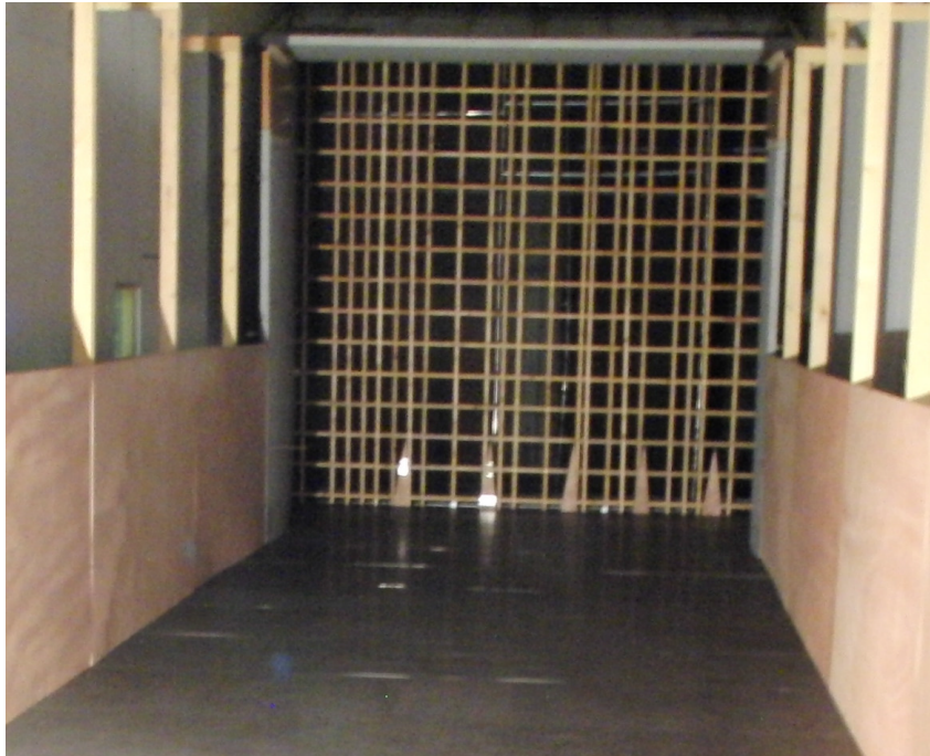
Figure 3.7 – Photo of the turbulence intensity grid placed at the return test section entry of Lucien Malavard wind tunnel.
