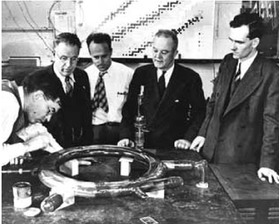
Figure 1.4: From left to right: Langmuir, Elder, Gurewitsch, Charlton and Pollock made the first observation of the SR light around the vacuum chamber of a 1947 general electric synchrotron. (Source: NSLS, Brookhaven)
